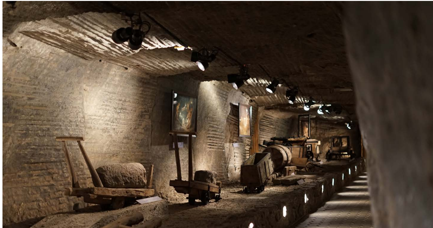
The Kraków Saltworks Museum in Wieliczka. A fragment of the permanent exhibition at the Kraków Saltworks Museum in Wieliczka. The exhibited equipment for horizontal and incline transport presents methods of delivering excavated material.
