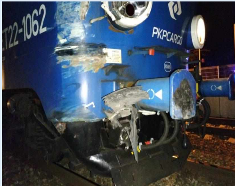
Photograph 19 – Consequences of the occurrence – damaged locomotive ET22-1062 (source: materials provided by the railway commission)
