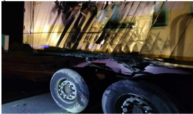
Photograph 18 – Consequences of the occurrence – damage sustained by the road tractor's semi-trailer (source: materials provided by the railway commission)
