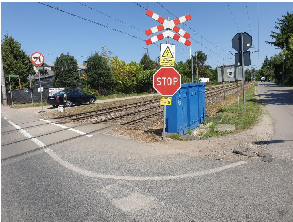
Photograph 4 - Visibility from 5 m from the left side of the level crossing to the right - situation as during the accident (source: PKBWK documentation)
