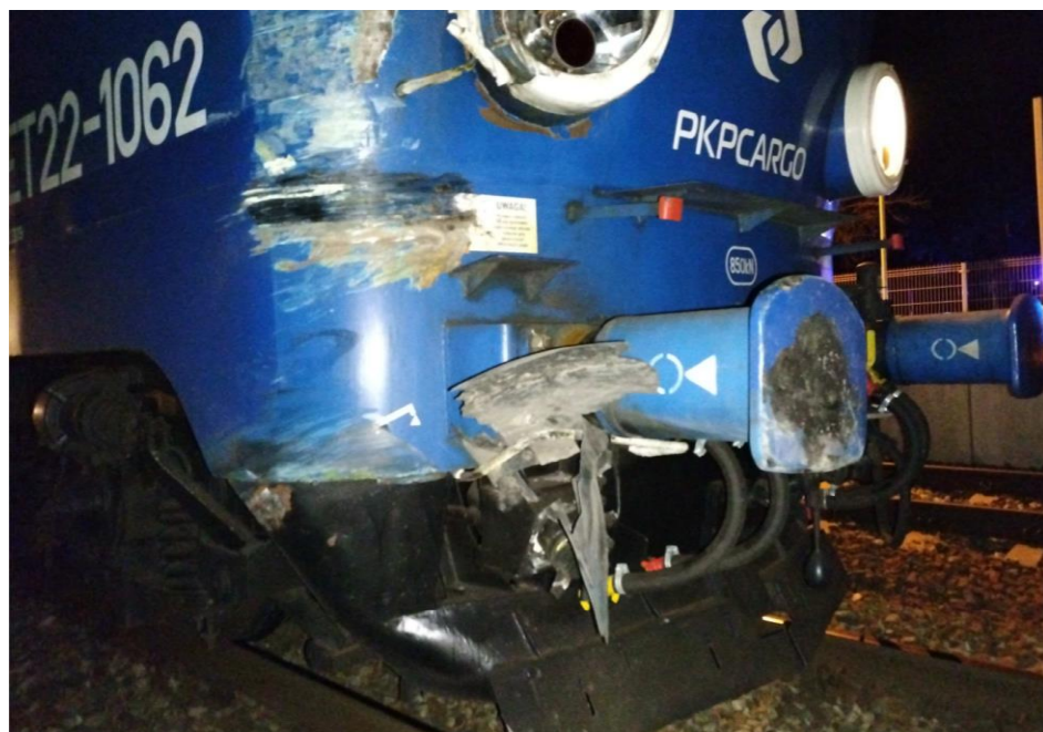
Photograph 10 – Damage sustained by the ET22-1062 locomotive (material provided by the railway commission)
