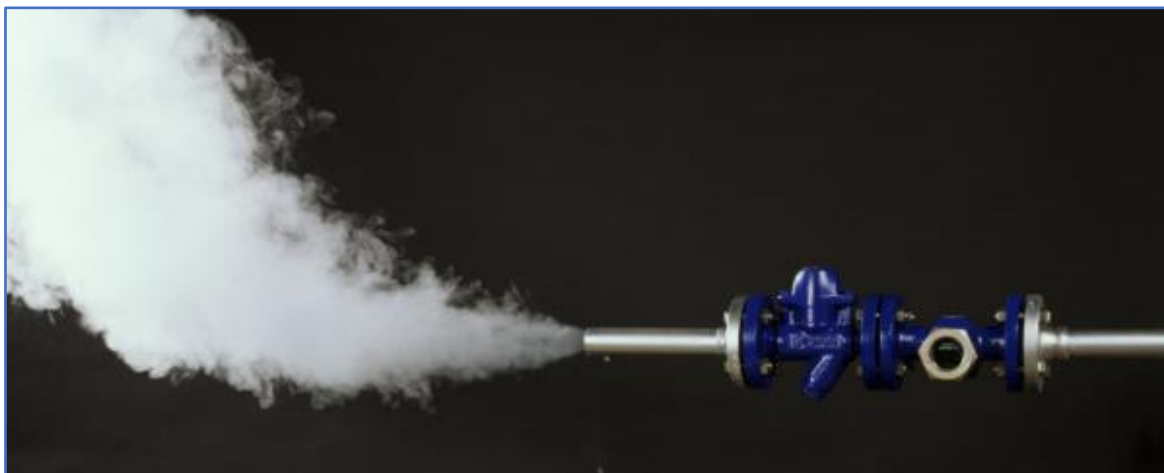
Pic. 1 Krzysztof Szalucki: only steam breaks through the trap
