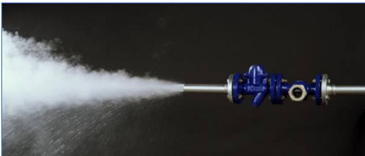
Pic. 2 Krzysztof Szalucki: partial condensate breakthrough through the trap
