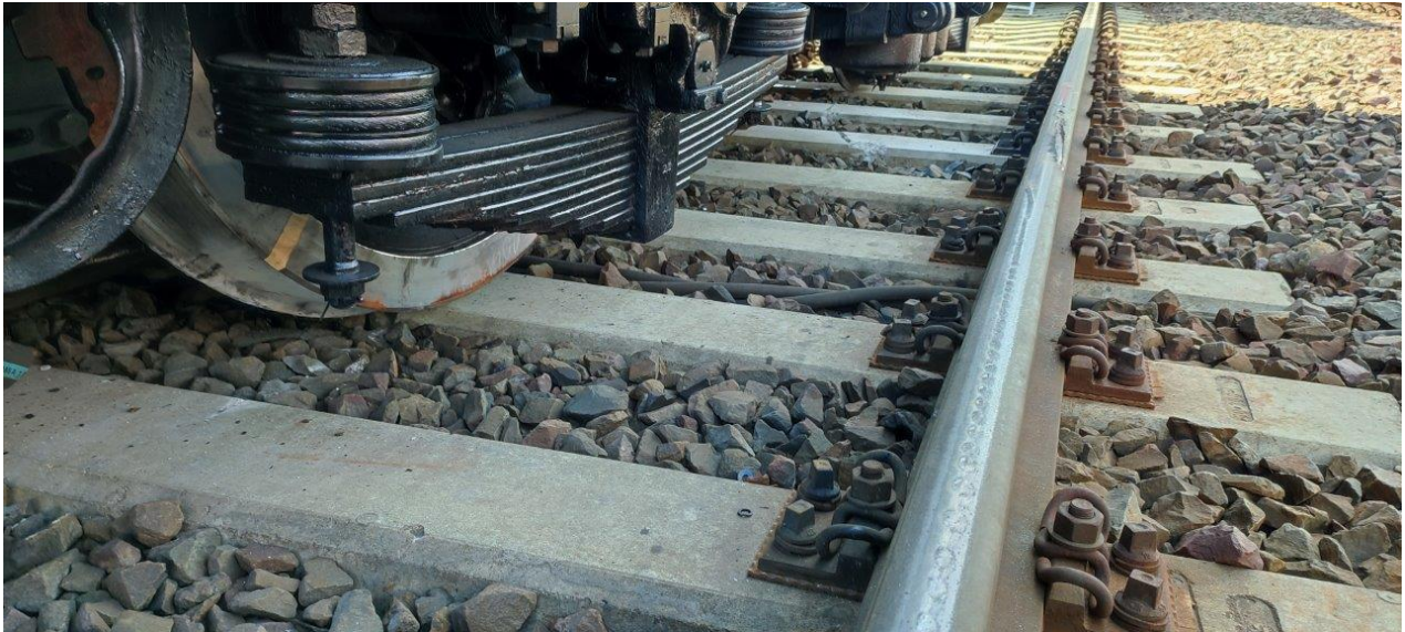
Photograph 4 - The place of derailment of the first wheelset of the first bogie (material provided by the railway commission)
