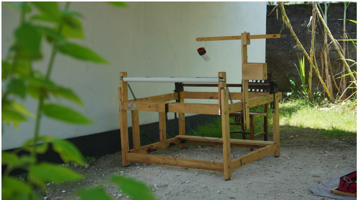
Putu Yuta, Kopernik | 19 September 2022, Jimbaran | A fully assembled ergonomic weaving tool in weaving mode
