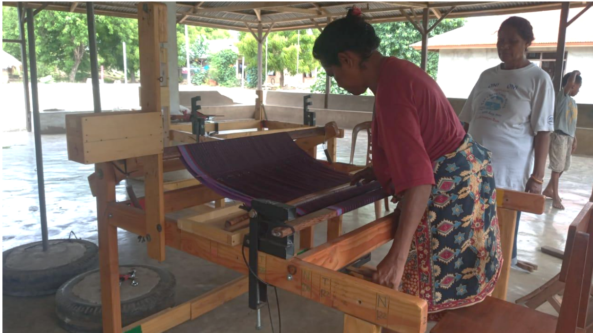
A weaver in Lembata is using the ergonomic weaving tool for weaving.
