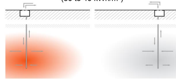
Aquifer thermal energy storage (ATES) (30 to 40 kWh/m 3 )
