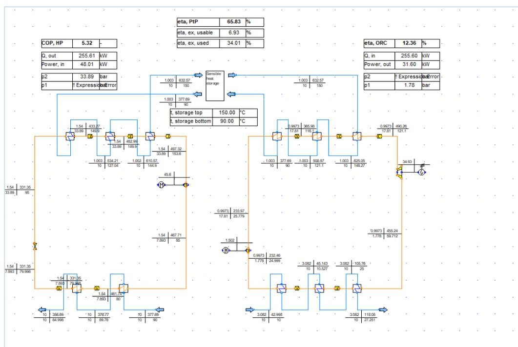
Figure 38: Illustration of the IPSEpro Carnot Battery model.
