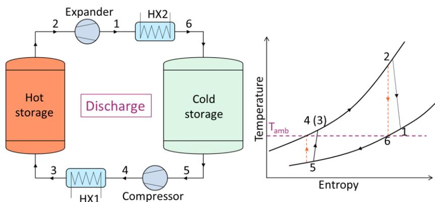
Figure 27: Discharge process diagram (left) and T-s diagram (right) of a Brayton battery.
