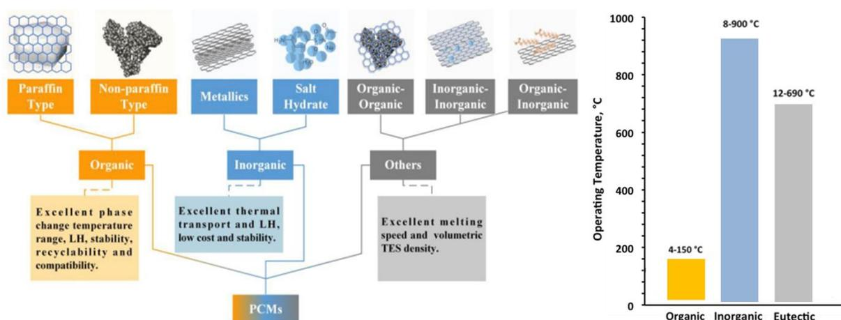
Figure 52: Different classes of phase change material and their advantages and disadvantages for thermal energy storage, as well as the respective temperature ranges for operation, based on [1], [11], [12].
