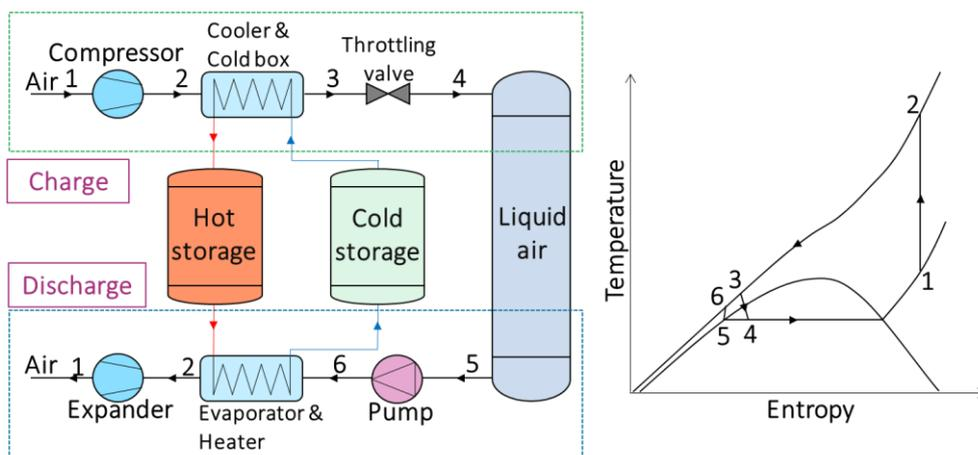
Figure 29: Charging and discharging process diagram (left) and T-s diagram (right) of the liquid air energy storage concept.
