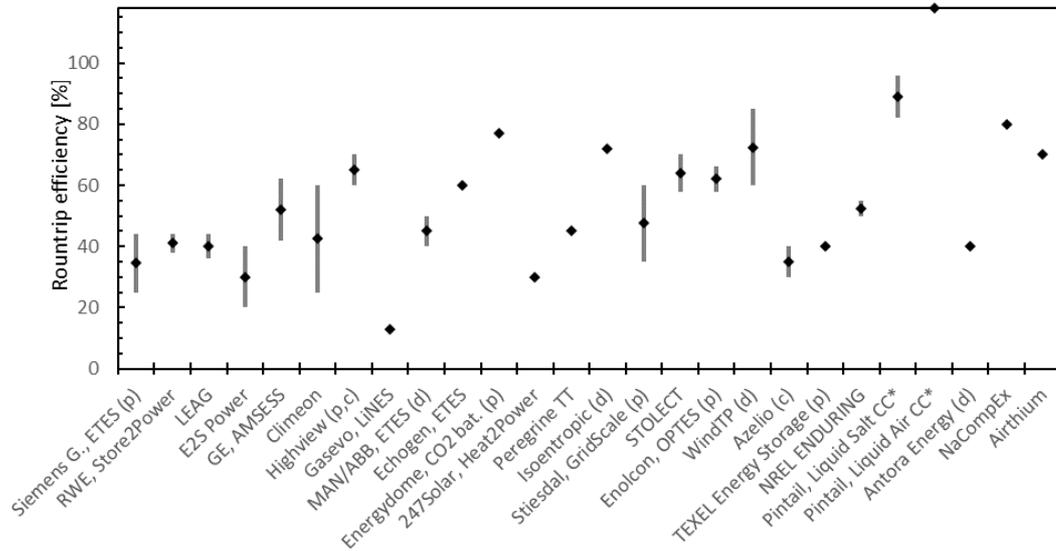
Figure 46: Overview of round-trip efficiency in the commercially CB systems (mostly declared as experimental values are limited). In notation (d) stands for demo, (p) pilot, (c) commercial units (built or under construction), \* for systems with additional fuel firing.
