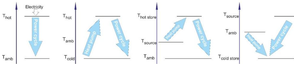
Figure 43: CB concept for thermal integration of heat sources and conversion systems [3].
