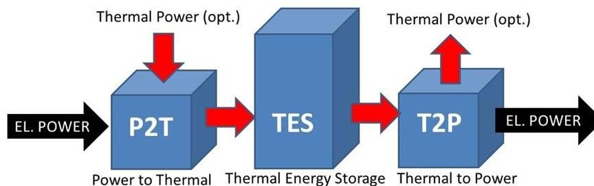
Figure 8: A simplified scheme of a typical Carnot Battery system.
