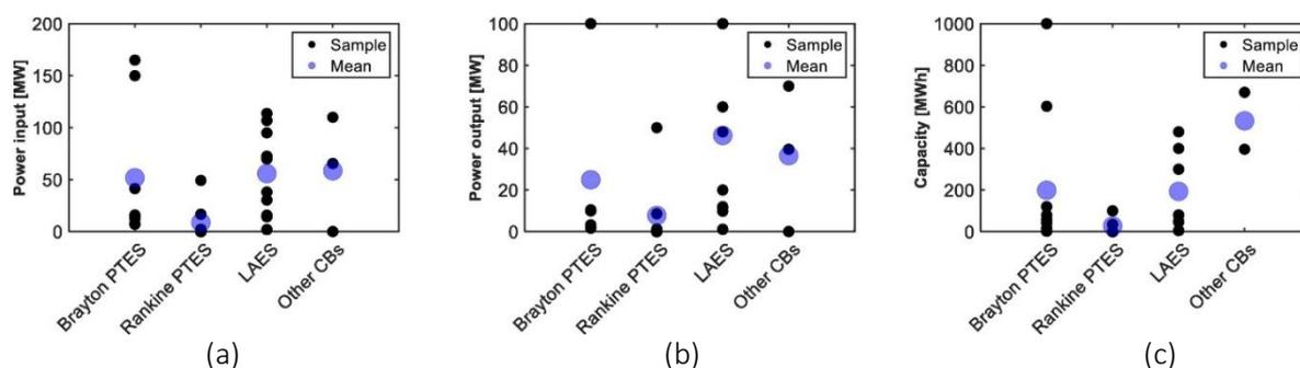
Figure 48: Storage systems performance from scientific studies regarding (a) power input, (b) power output and (c) system capacity [4].
