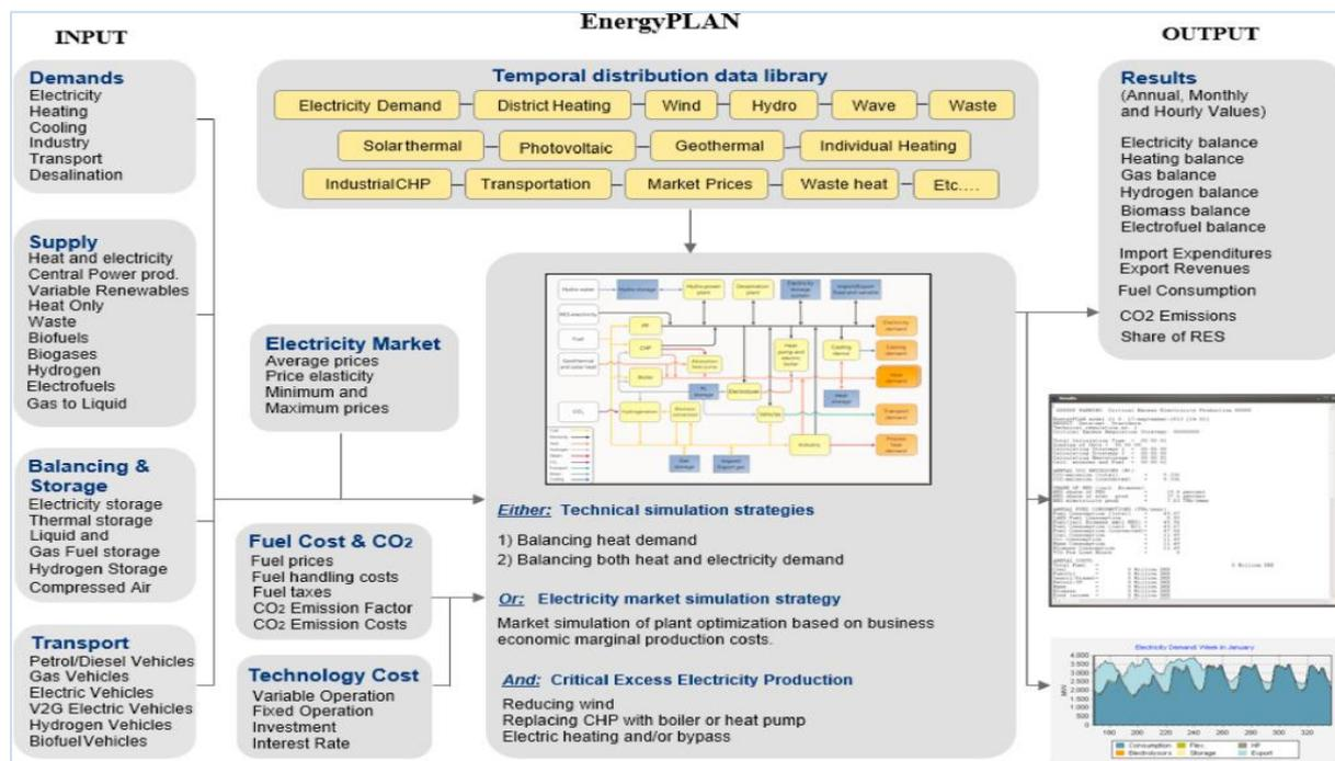
Figure 40: Illustration of the EnergyPLAN model developed by AAU.
