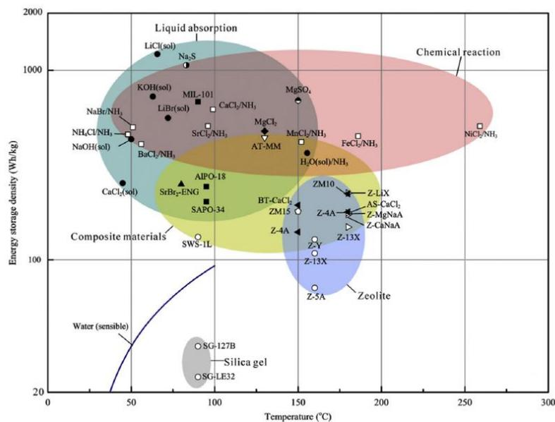
Figure 54: Overview of common thermochemical reactant pairs, their associated temperature levels and energy storage densities. Based on [14].
