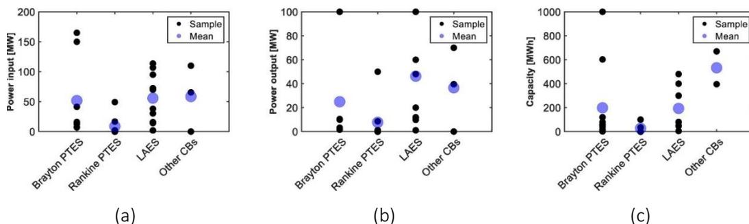
Figure 14: Storage systems performance from scientific studies regarding (a) power input, (b) power output and (c) system capacity<sup>9</sup>.
