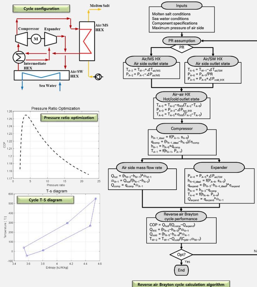
Key illustrations: cycle configuration, calculation algorithm, model results
