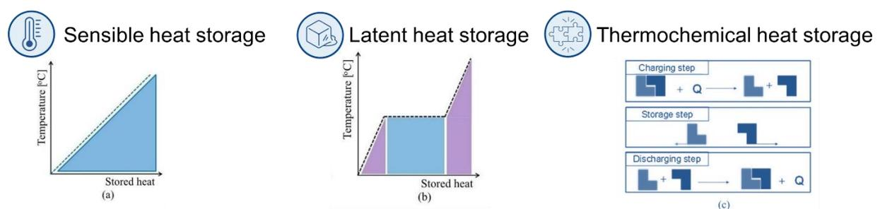
Figure 50: Methods of thermal energy storage: (a) sensible heat; (b) latent heat; (c) thermo-chemical, based on [4].
