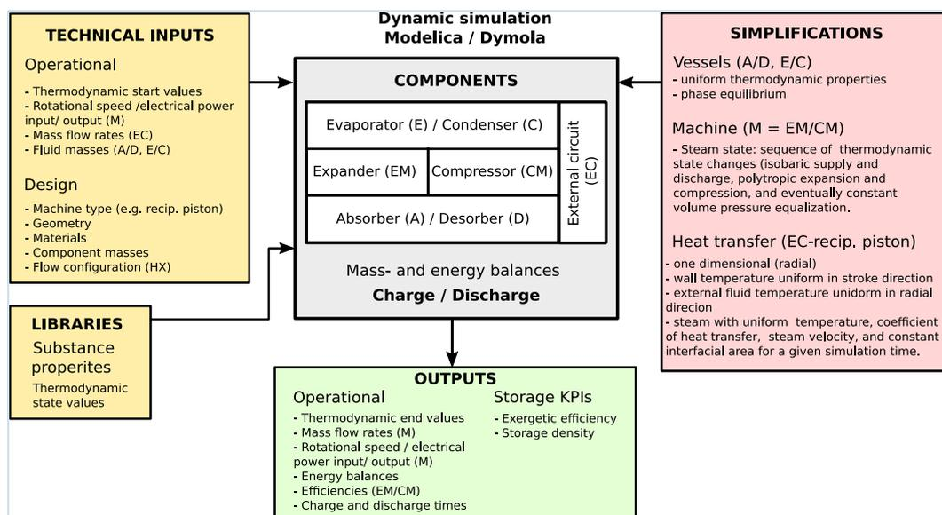
Figure 37: Simplified model structure of the Lamm-Honigmann system. Main components, inputs, simplifications, and outputs.
