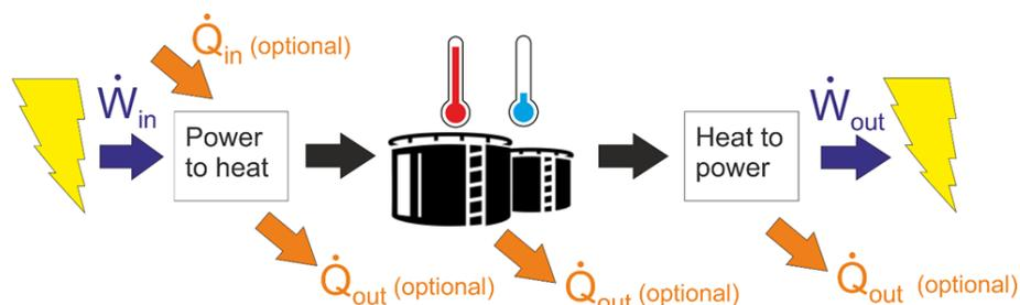
Figure 9: General principle of Carnot Battery systems.
