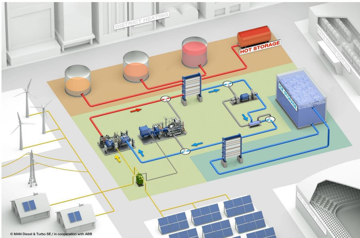
Figure 53: Schematic of the MAN ETES System by MAN Energy Solutions, based on [13].
