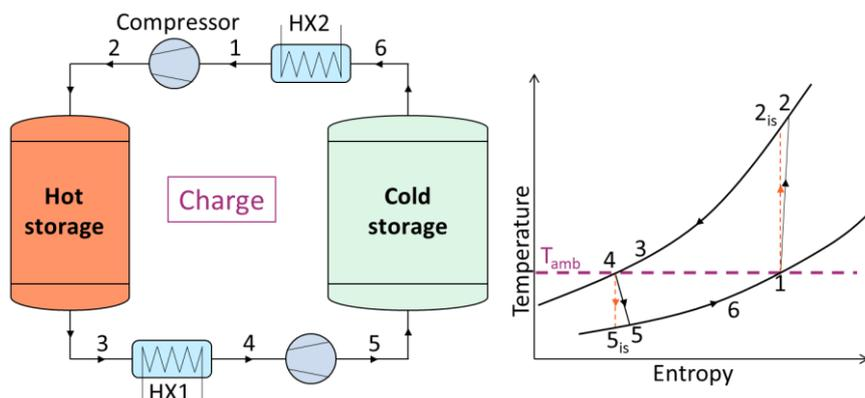
Figure 26: Charging process diagram (left) and T-s diagram (right) of a Brayton battery.
