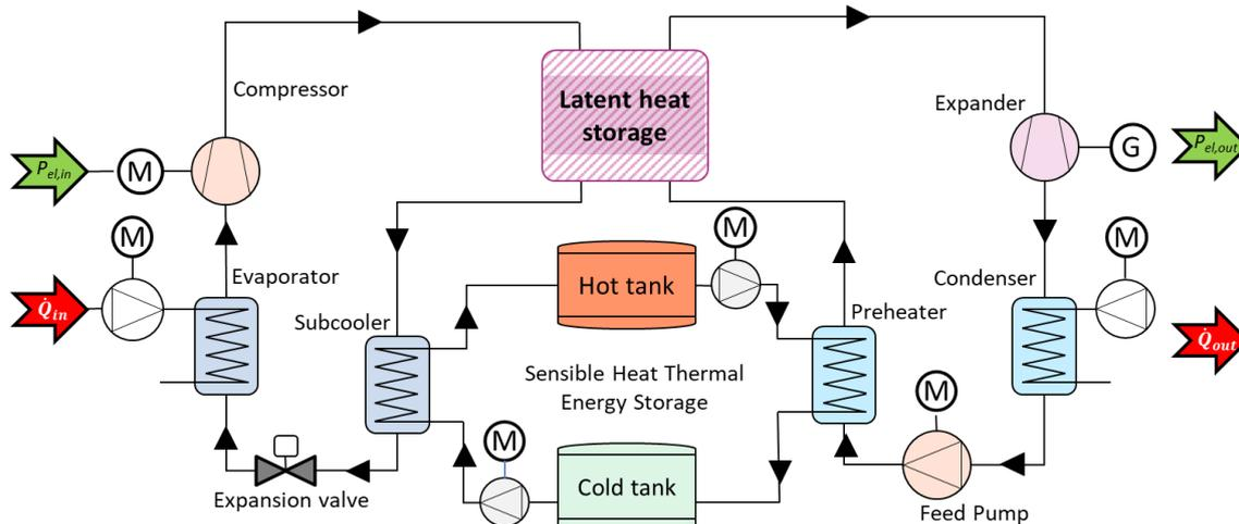
Figure 24: Simplified laboratory diagram of the CHESTER installation.
