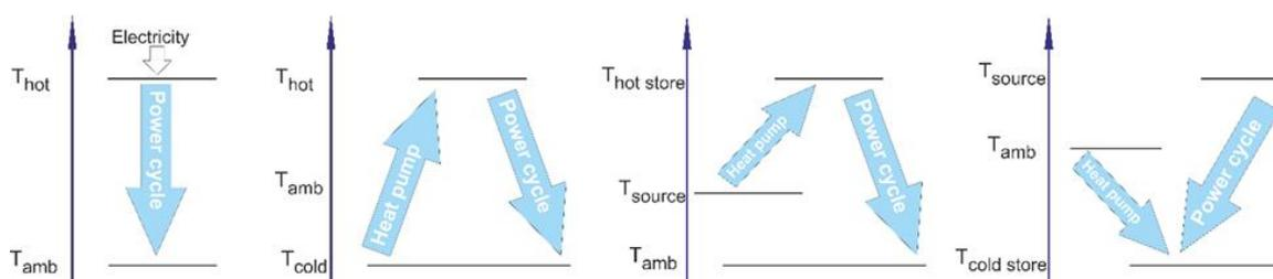
Figure 10: CB concept for thermal integration of heat sources and conversion systems.
