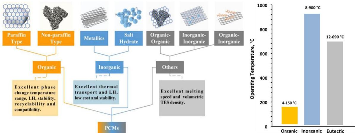
Figure 17: Different classes of phase change material and their advantages and disadvantages for thermal energy storage, as well as the respective temperature ranges for operation, based on Dumont et al., 2020<sup>4</sup>; Maha, 2021<sup>17</sup>; Qiu et al., 2019<sup>18</sup>.
