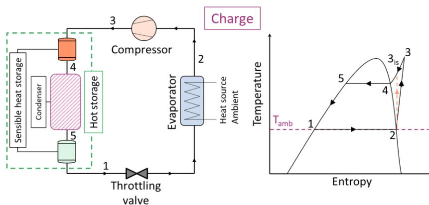
Figure 22: Scheme of the charging process of a Rankine based Carnot Battery (left) and the associated T-s diagram (right).
