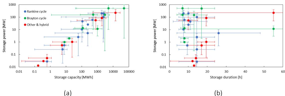
Figure 12: Storage power output and capacity (a) and discharge duration (b) for the commercially developed CB systems.
