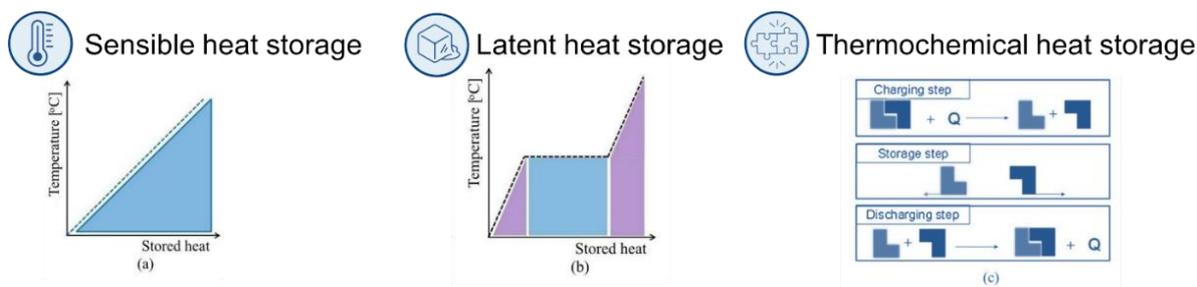
Figure 15: Methods for thermal energy storage: (a) sensible heat; (b) latent heat; (c) thermo-chemical, based on Sarbu & Sebarchievici, 2018<sup>11</sup>.
