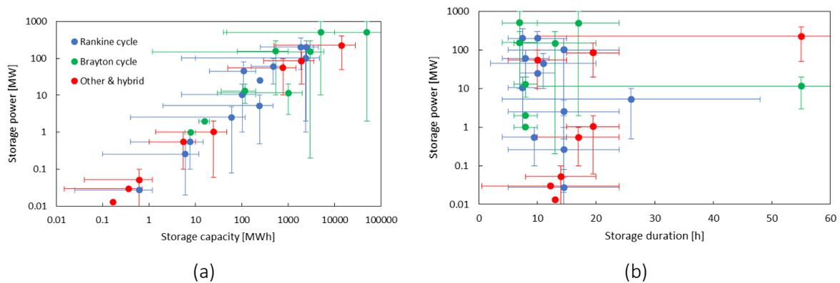
Figure 45: Storage power output and capacity (a) and discharge duration (b) for the commercially developed CB systems.
