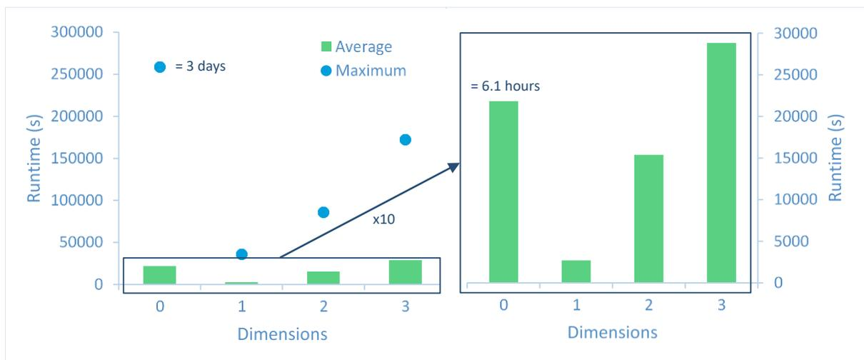
Figure 33: Average and maximum runtime of models categorized by dimensions considered by each model. The total numbers of considered models per dimension were 7 for 0-D, 15 for 1-D, 7 for 2-D and 3 for 3-D.
