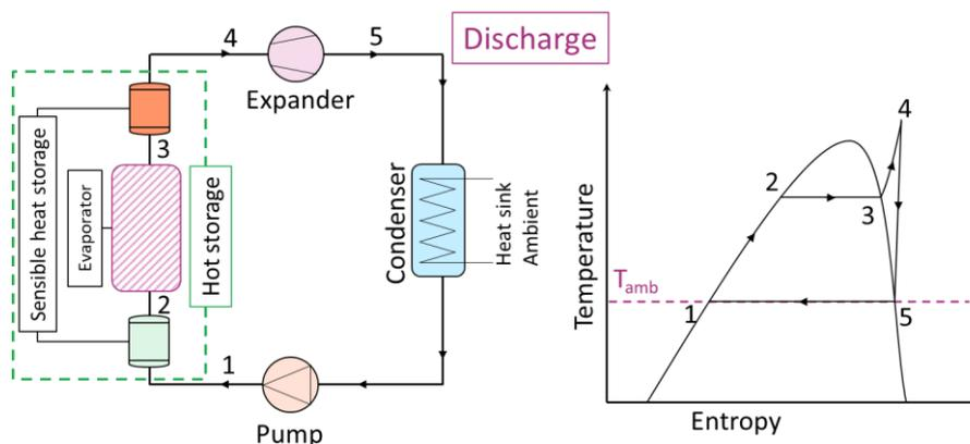
Figure 23: Simplified scheme of the discharging process of a Rankine based Carnot Battery (left) and the associated T-s diagram (right).
