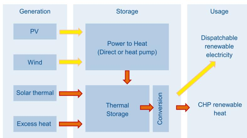
Figure 49: Basic working principle of a Carnot Battery, divided into the three sections Generation, Storage and Usage. Yellow arrows indicate electrical energy, red arrows thermal energy (heat or cold). Source: AEE INTEC.
