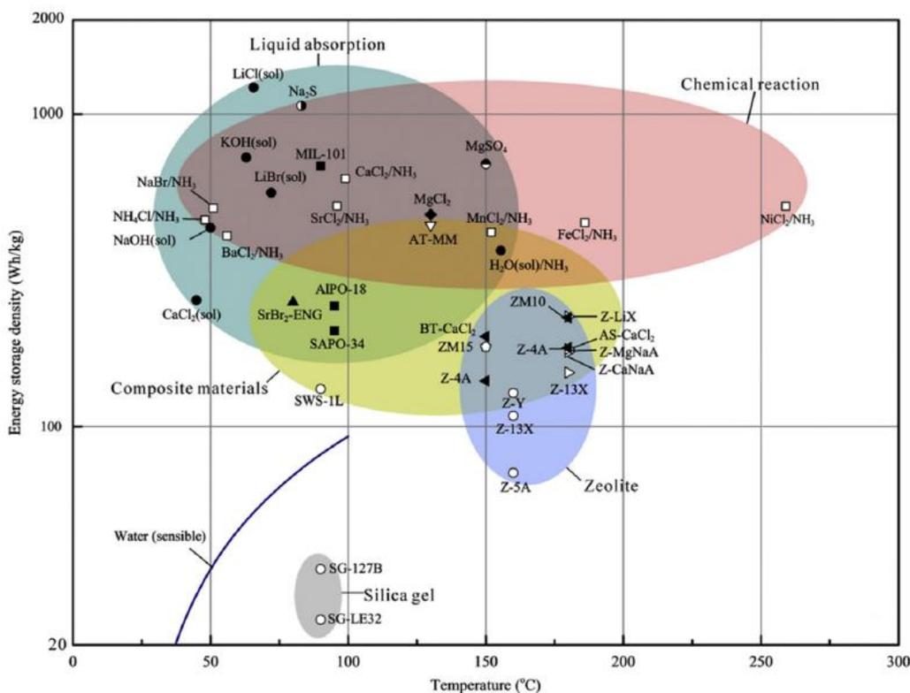
Figure 18: Overview of common thermochemical reactant pairs, their associated temperature levels and energy storage densities. Based on Aydin et al., 2015<sup>19</sup>.
