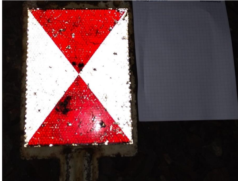
Photograph 4. The train end signal used on train TME 684013 (next to it is a non-reflective sheet of white paper for comparison)
