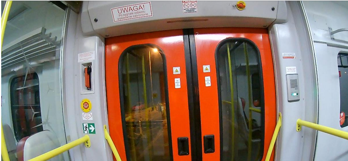
Photo 7 - View from inside the vehicle of the installed intercom at the front door (vehicle monitoring).
