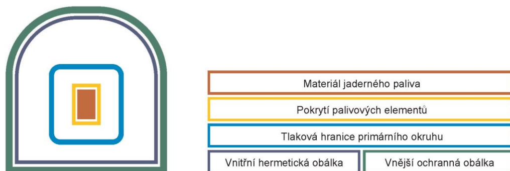
Fig. B.10: Schematic Diagram of the Physical Barriers
