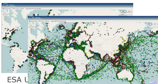
Ships monitored by a) terrestrial AIS b) terrestrial and Sat-AIS (source: Exact Earth)
