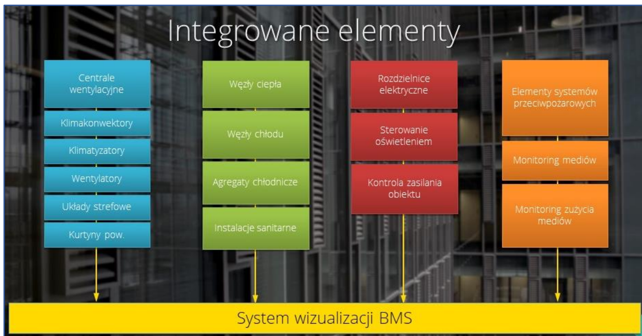
fot. 1 I-MATIC: Building Management System
