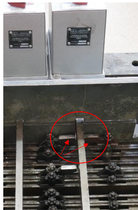
Photograph 2 – View of the combiner with UZE-02 electromagnetic locks on the dependent box Gg2
