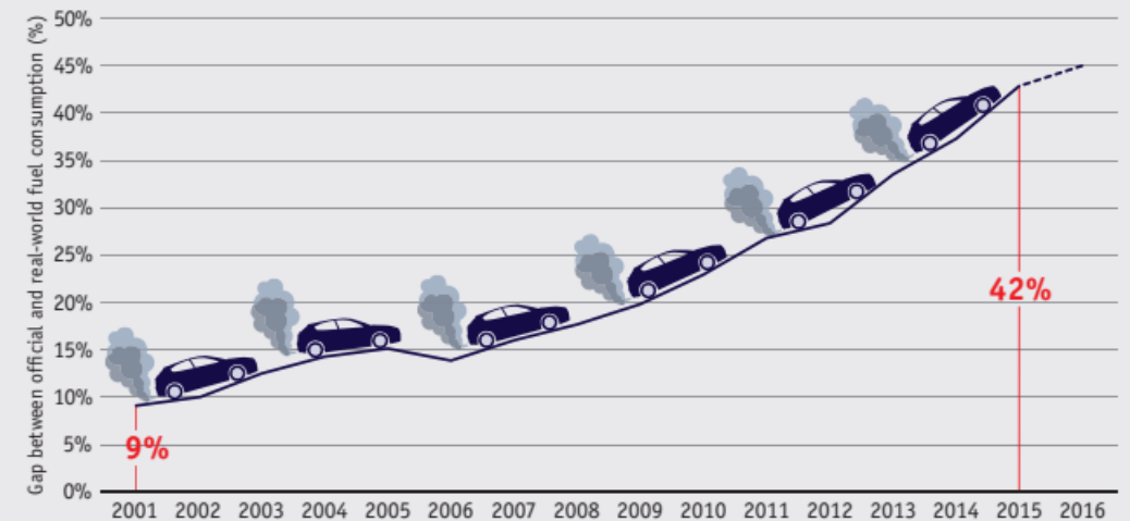
Average divergence between official and real-world fuel consumption of new passenger cars
