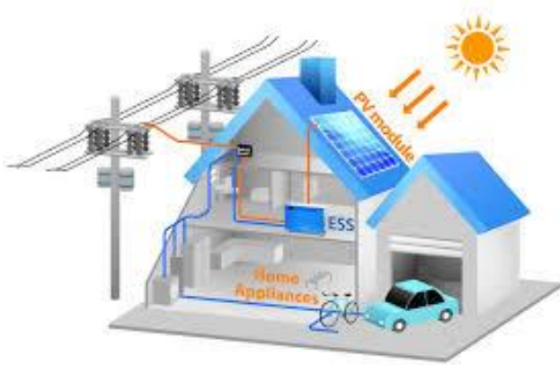
Figure 30 - The Prosumer concept. The Power transmission goes from one-way to two-way lines
