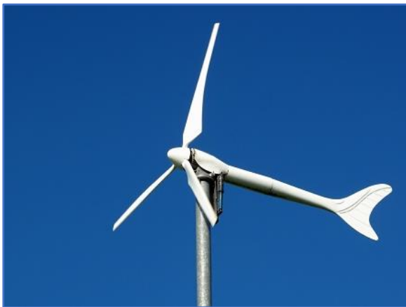
Pic. 1 ekolhouse: three blade horizontal axis wind turbine
