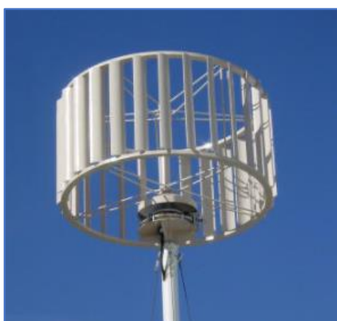
Pic. 8 instsani: drum vertical wind turbine
