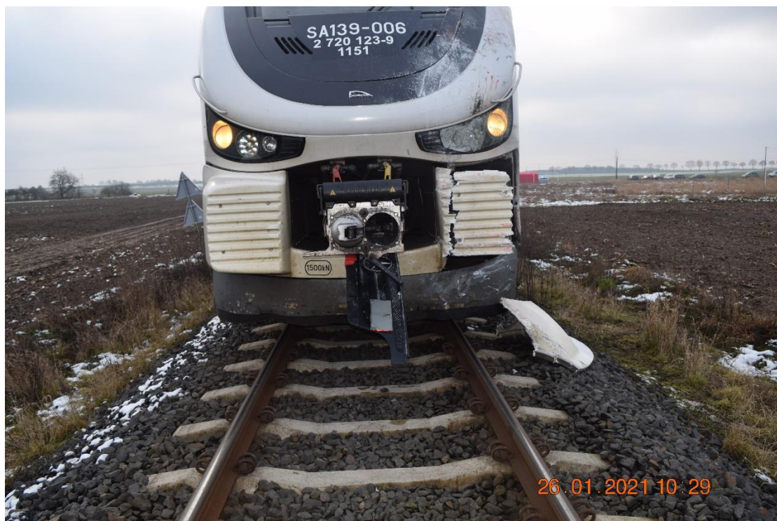
Photo 5- View of damage to the front of a railway vehicle after an accident
