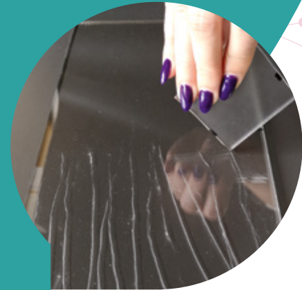
Photo on the left (upper part) - glass with a hardening coating (diamond-like). Photo on the left (bottom part) - glass without a coating.
