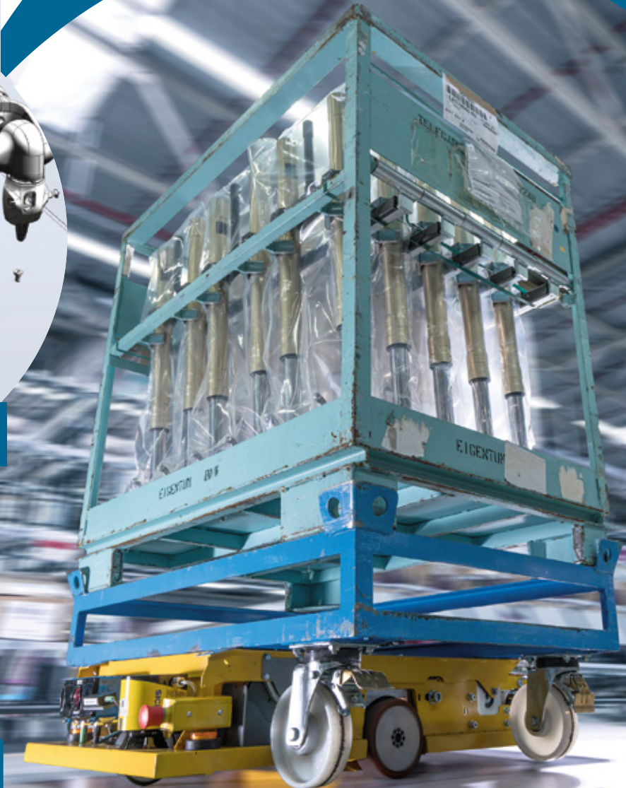
The BMW GROUP's Smart Transport Robot for automated commissioning of sequence racks. Source: BMW GROUP.
