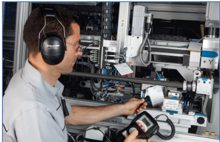
Pic. 2 Festo: detecting air leakage using acoustics
