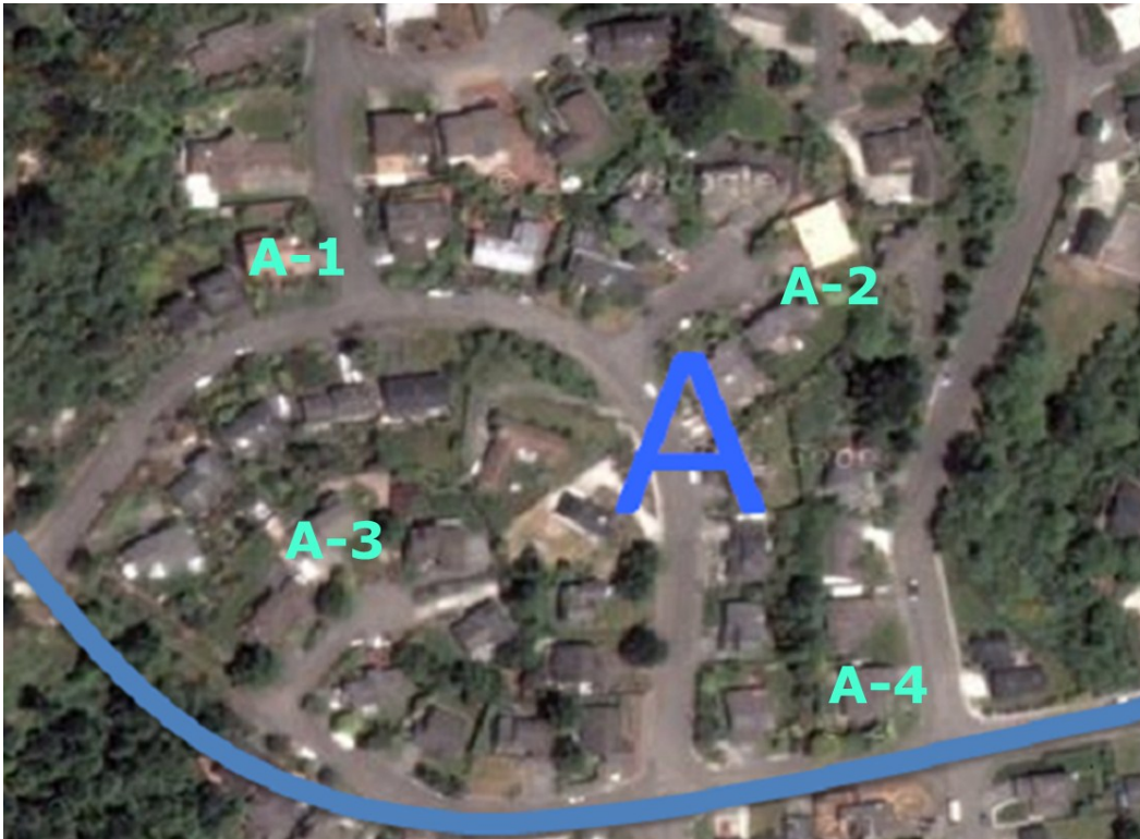
Figure 9: As potential rescue sites are identified, they are numbered and added to the Sector letter to produce a unique Worksite ID for each site.
