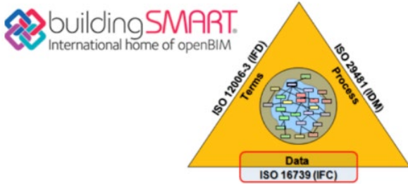
Figure 56: Structure of format, dictionary and information exchange methods in an Open BIM environment. 154
