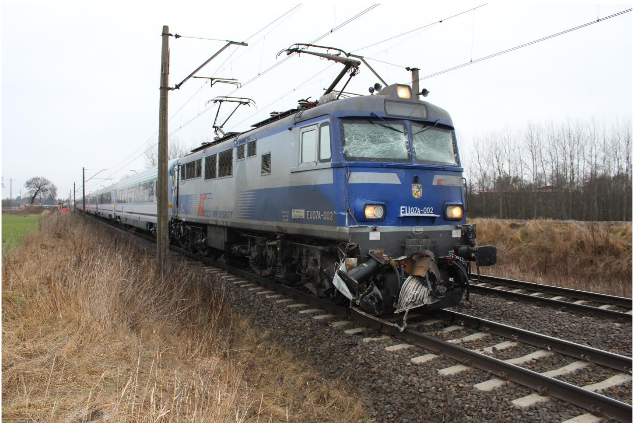
Fig. 4 - View of the railway vehicle after the accident
