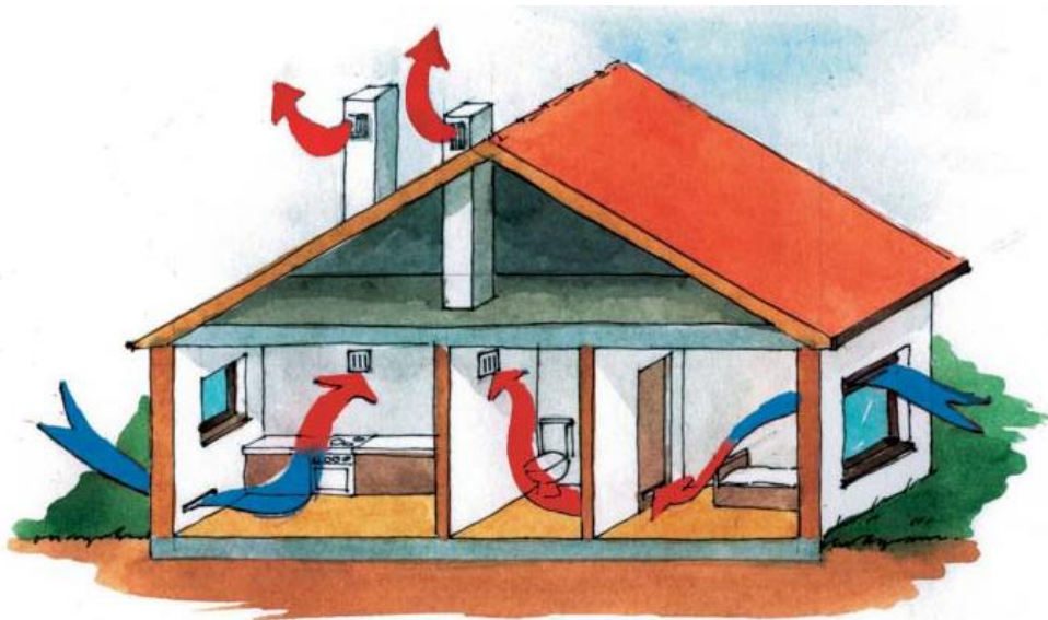
Pic. 1 budujemydom: diagram illustrating gravitational ventilation
