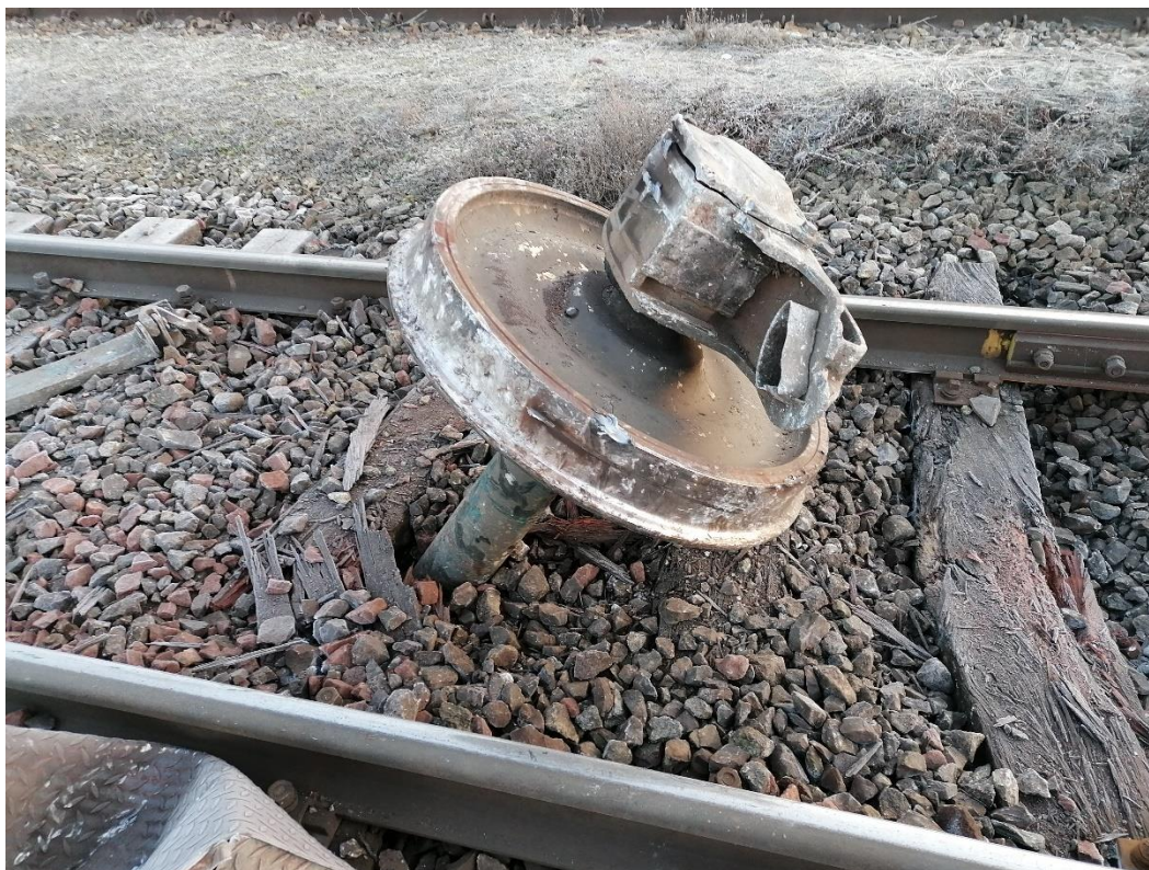
Photograph 2 - A view of one part of the broken axle (source: materials provided by the railway commission)
