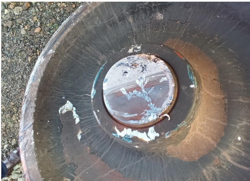
Photograph 6 - A view of the broken axle (material provided by the railway commission)
