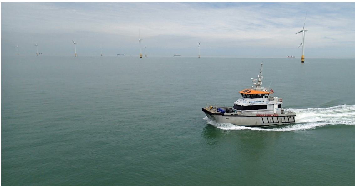
Figure 71. Example of crew transfer vessel (Photo: Göran Loman).
