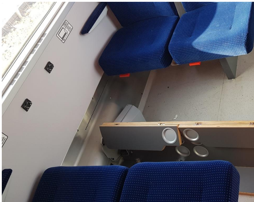
Photo 3 – broken table in the passenger coach (photo by PKBWK)
