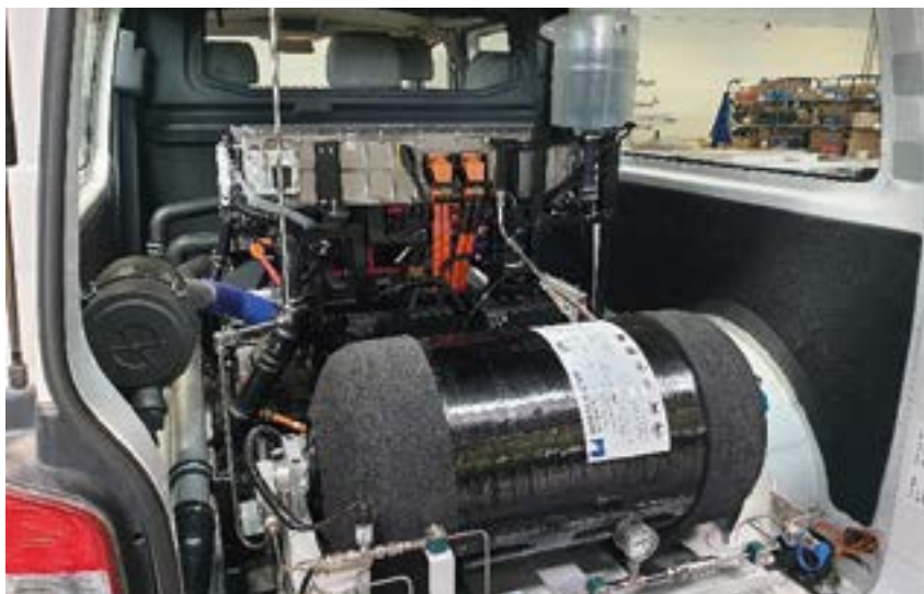
■ Hydrogen tank installed in a delivery vehicle
