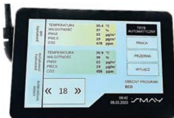
■ Room controller designed for classrooms and ancillary premises
