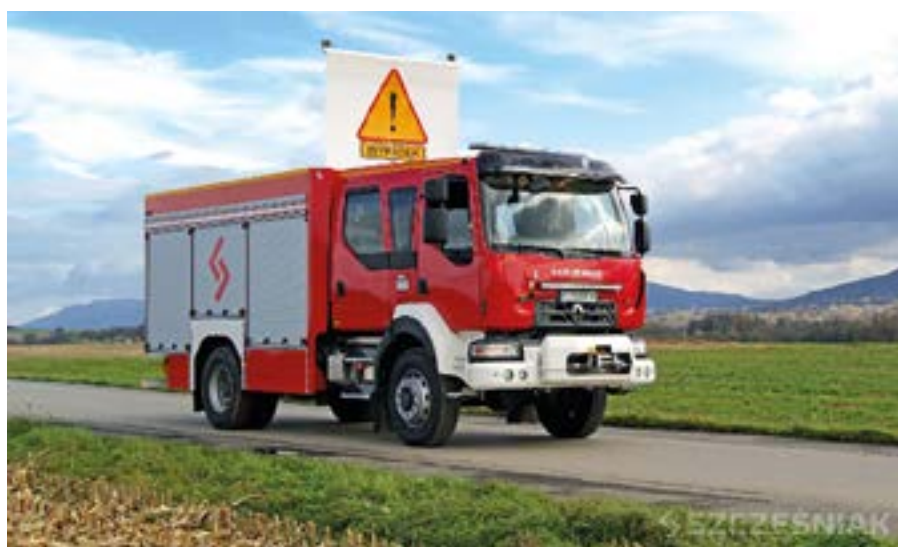
■ The prototype of a medium-sized rescue and fire-fighting vehicle on the Renault D16 4x4 chassis
