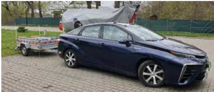
■ Hydrogen tank connected to a passenger car (Toyota Mirai) during a test
