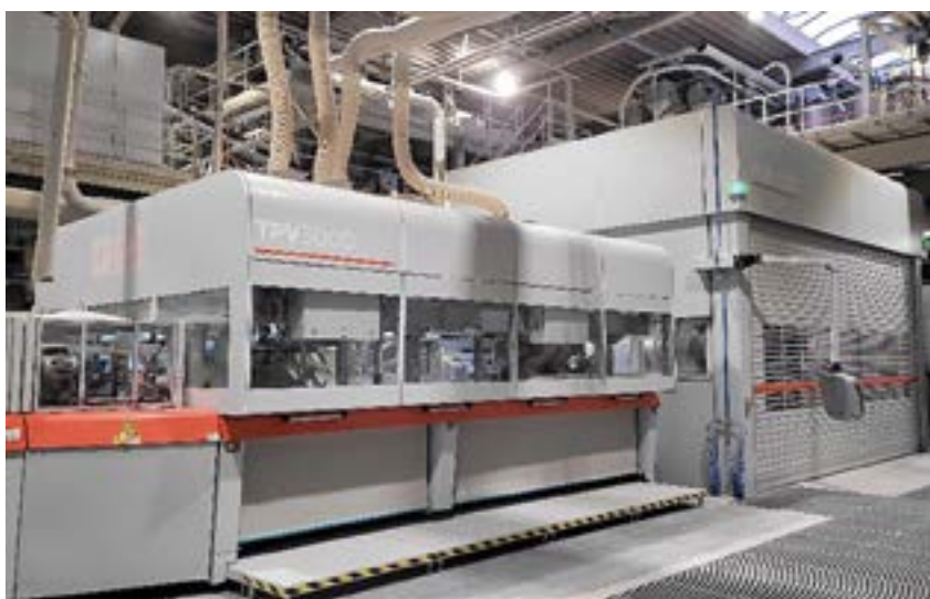
■ TPV3000 cutter and PCR3000 press as central elements of a line for the production of large-format slabs
