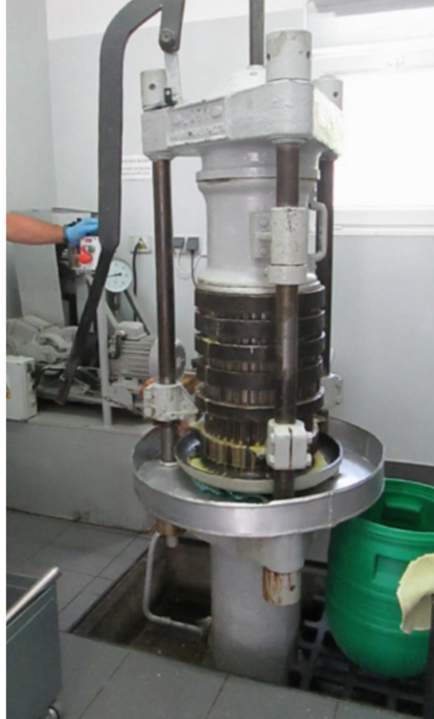
Pressing device used for pressing oil from the gold-of-pleasure seeds, Photo: Agnieszka Staniszweska
