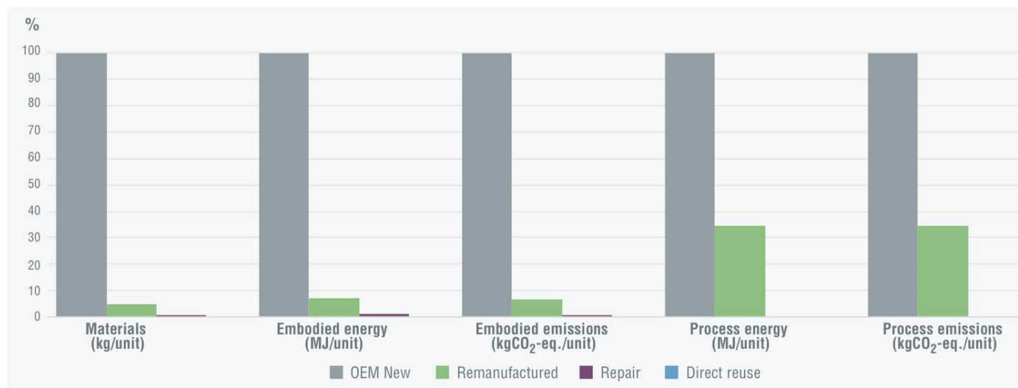
Figure 22: Comparative weighted average impacts per unit for US via value-retention processes for vehicle parts production with 100 per cent cast iron engines
