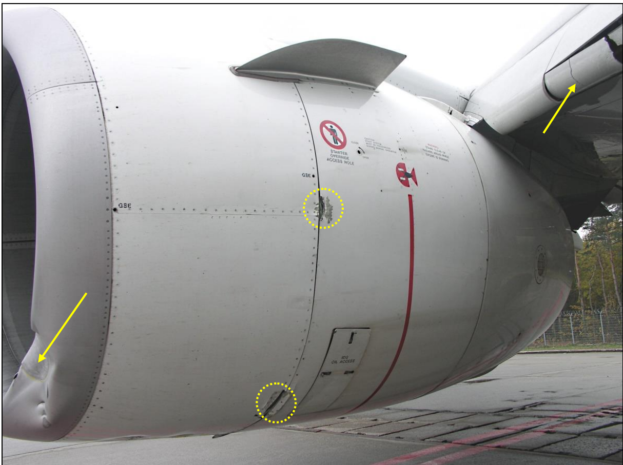
69 – Damage to the left side of the right engine nacelle. Marked damage resulting from a collision with a light and damage to the Krüger flap
