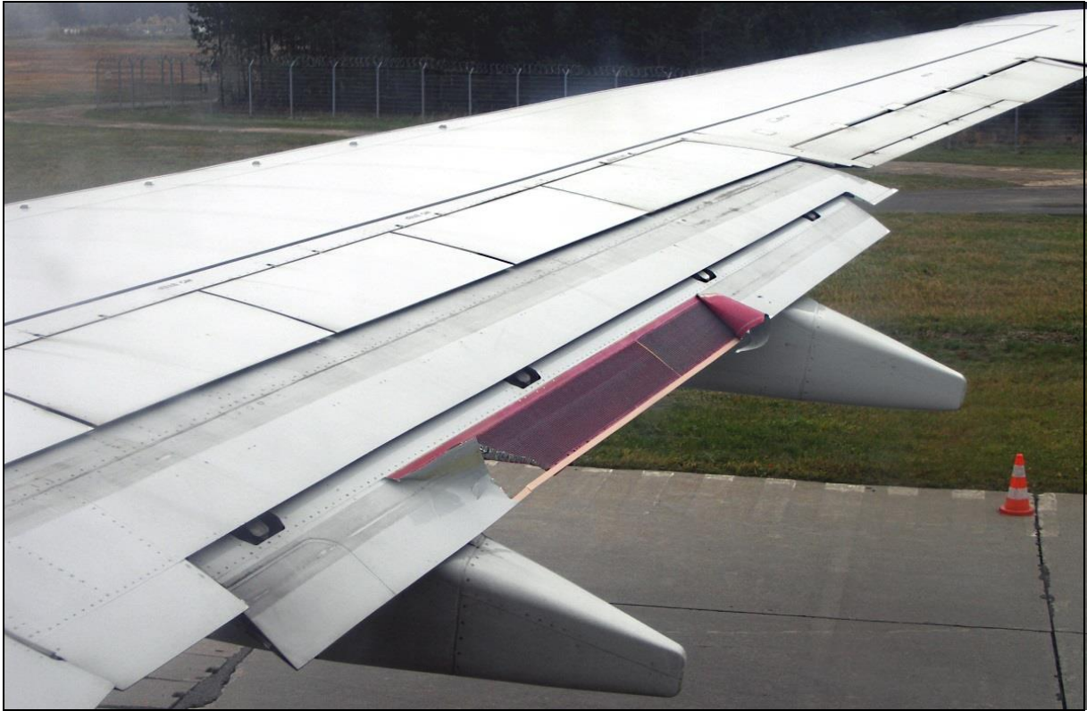
78 – Damage to the right outboard flap – top view
