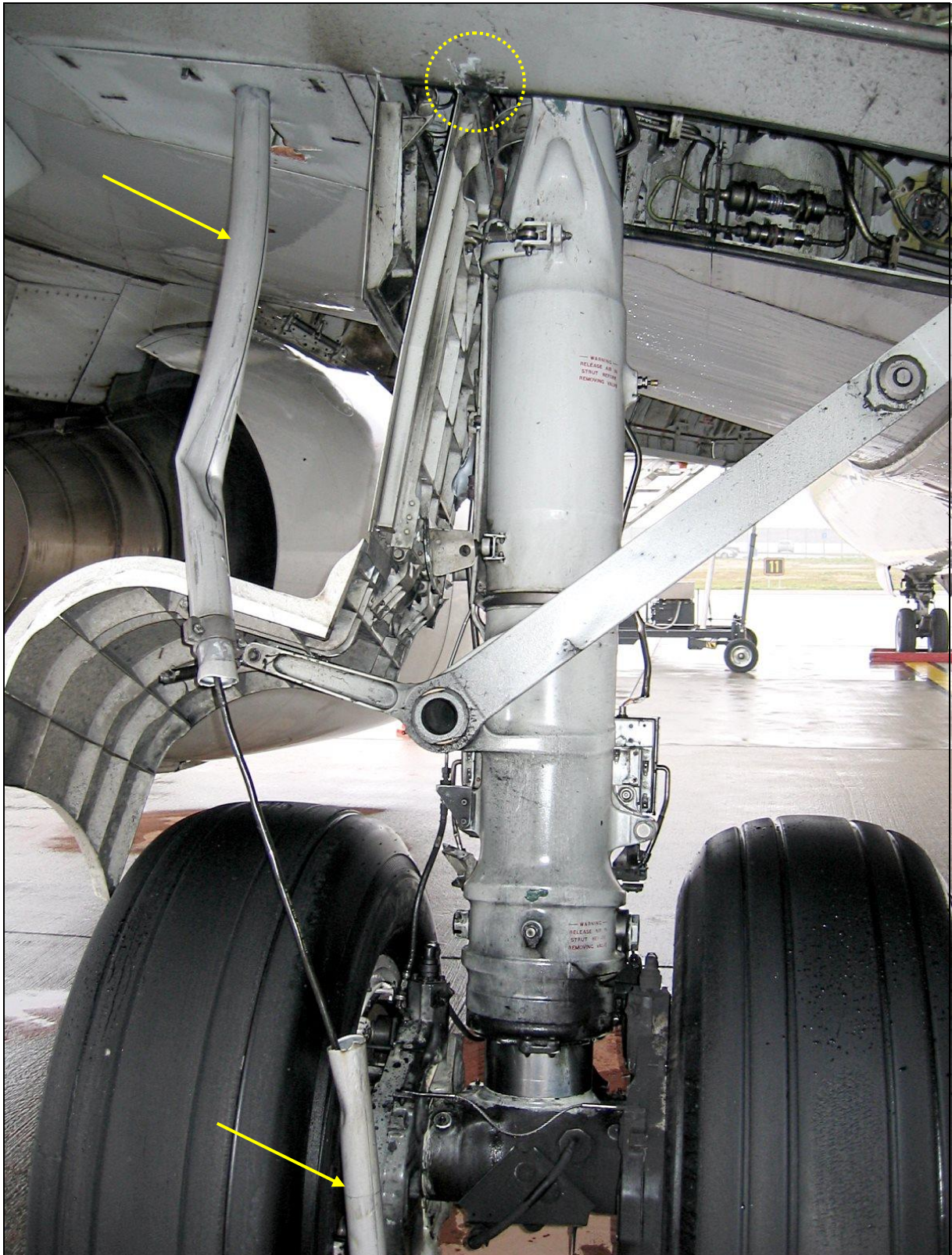
58 – Damage to the rear section of the left main landing gear door. Arrows show the lights pieces stuck in the airplane structure [photo: airplane crew]
