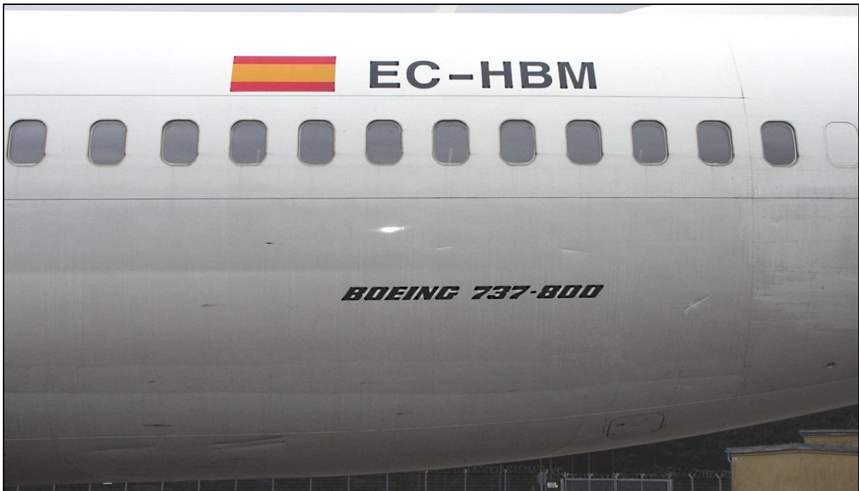
81 – Scratches and abrasions of the left rear part of the fuselage skin
