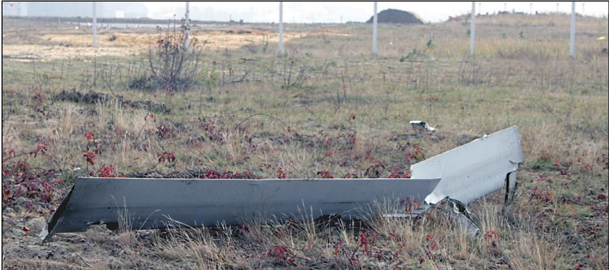
13 – Trailing part of the left outboard flap separated from the airplane
