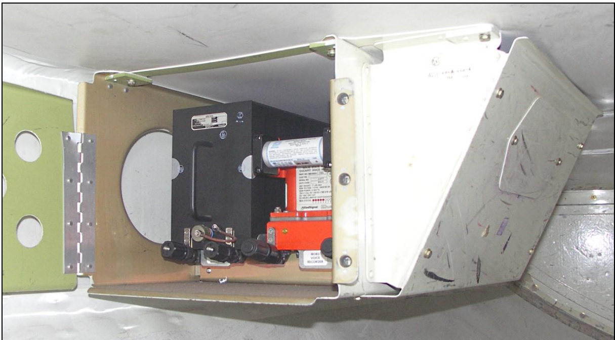
39 – Cockpit Voice Recorder prior to removal from the airplane
