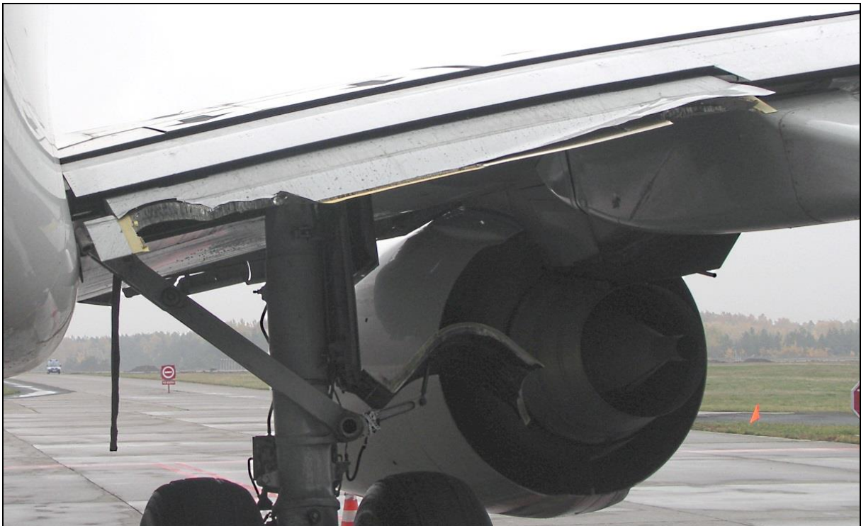
73 – Damage to the left inboard flap, rear view
