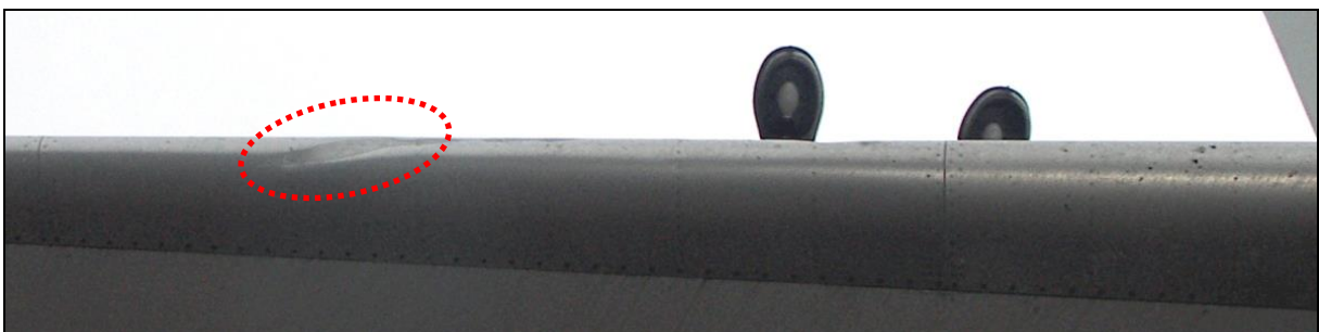
93 – Damage to the right horizontal stabilizer leading edge – close-up
