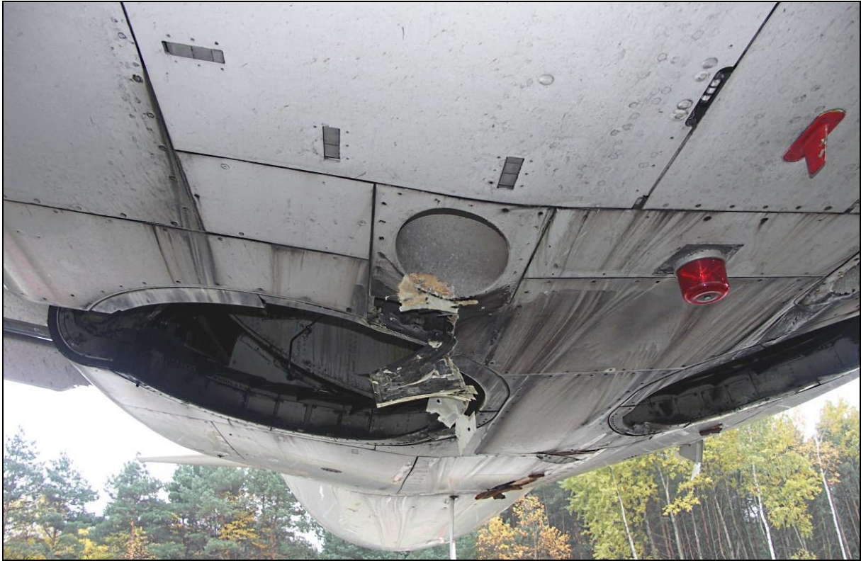
86 – Damage to the belly fairing – close-up
