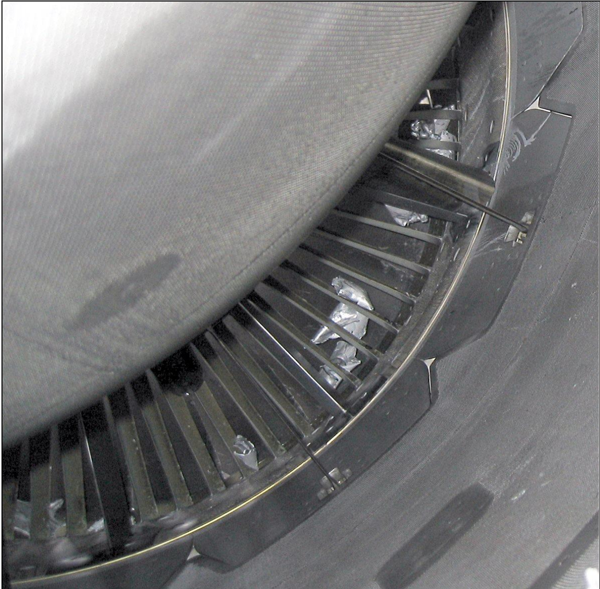
76 – Lights pieces, which went through the outer flow of the engine [photo: airplane crew]
