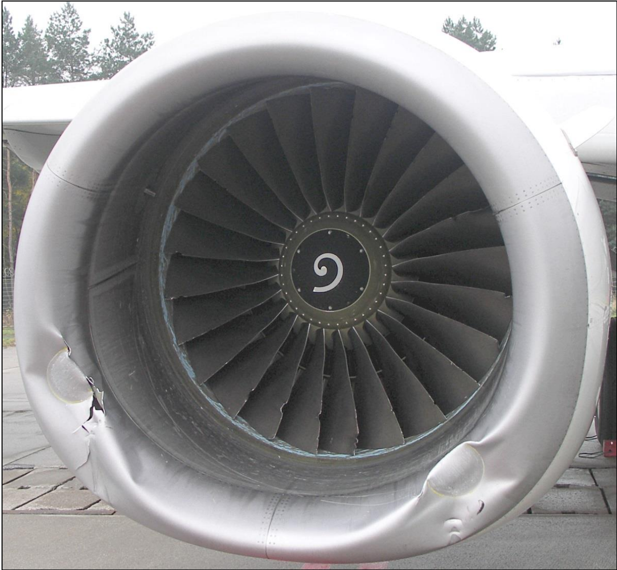
70 – Damage to the right engine inlet
