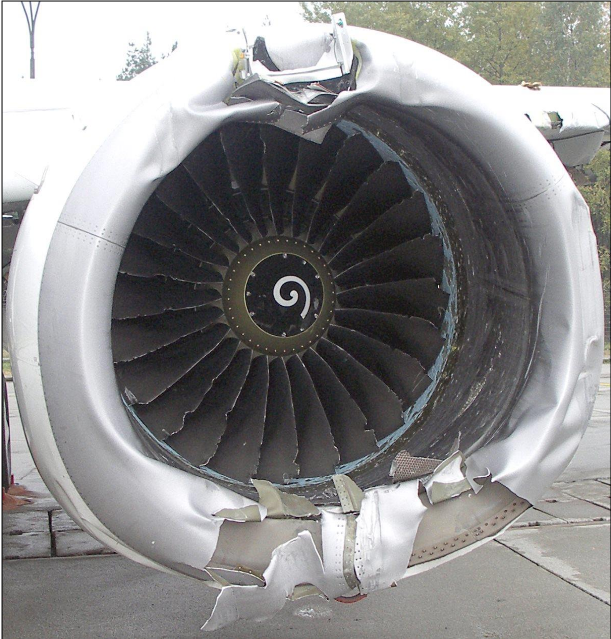
49 – Left engine inlet – visible damage
