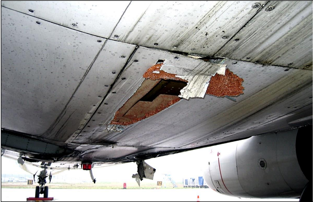
88 – Damage to the belly fairing – close-up [photo: airplane crew]
