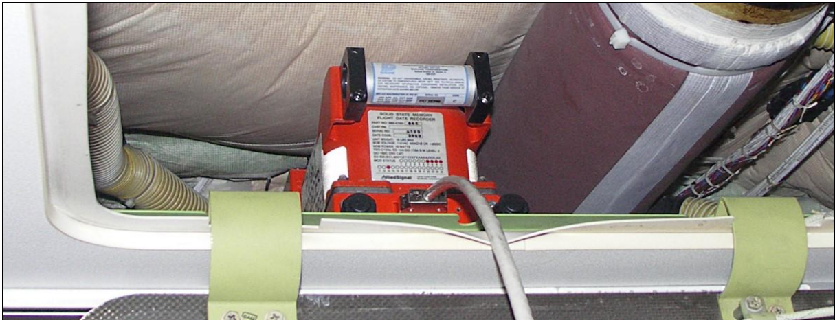
38 – Flight Data Recorder prior to removal from the airplane
