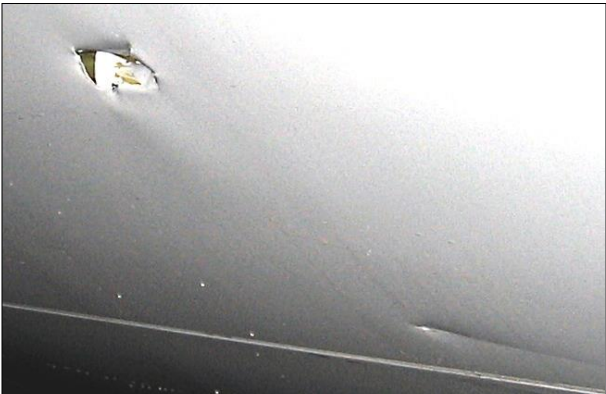
67 – Puncture and scratch of the fuselage – close-up [photo: airplane crew]
