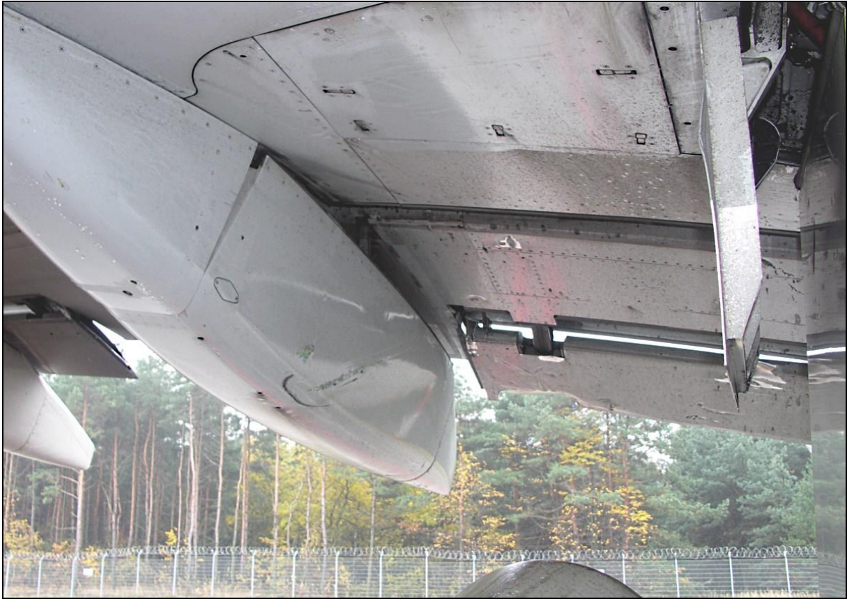
80 – Damage to the right inboard flap – bottom view
