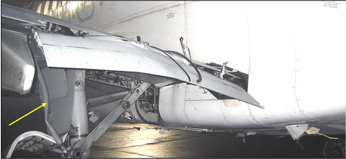
59 – Damage to the left main landing gear door and the left inboard flap. Arrows show the lights pieces stuck in the airplane structure [photo: airplane crew]
