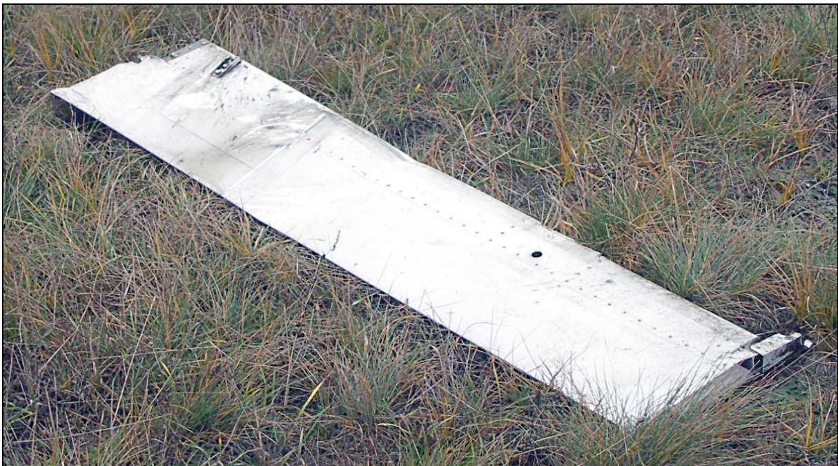
14 – Trailing part of the right outboard flap separated from the airplane
