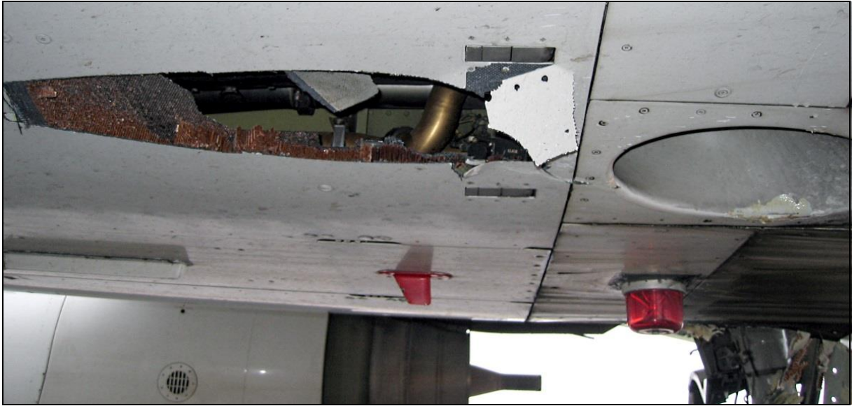
84 – Damage to the belly fairing – close-up [photo: airplane crew]
