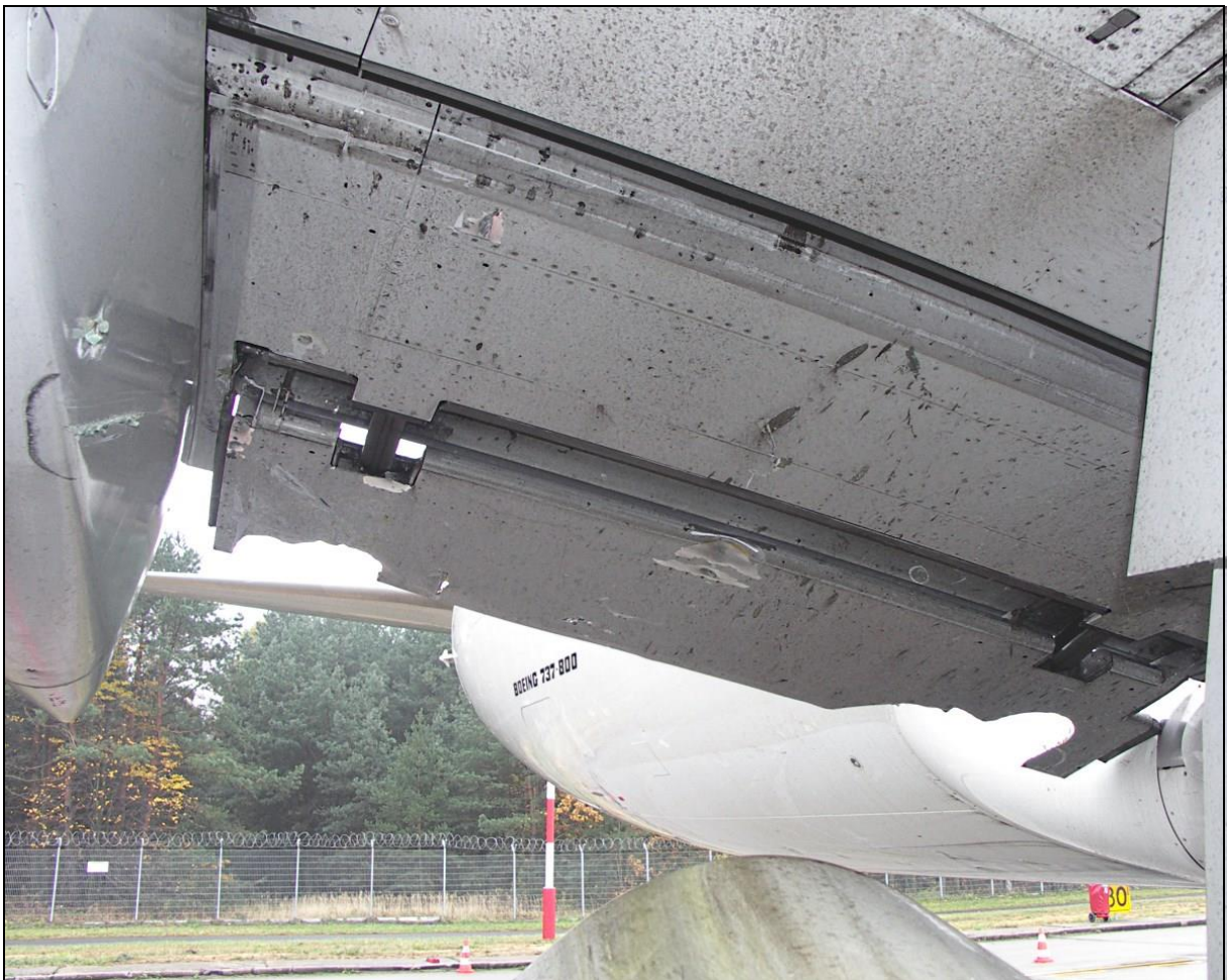
79 – Damage to the right inboard flap – bottom view
