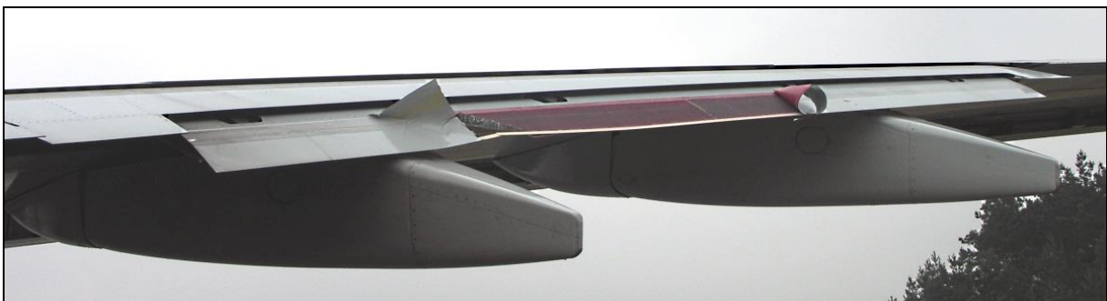
77 – Damage to the right outboard flap – rear view
