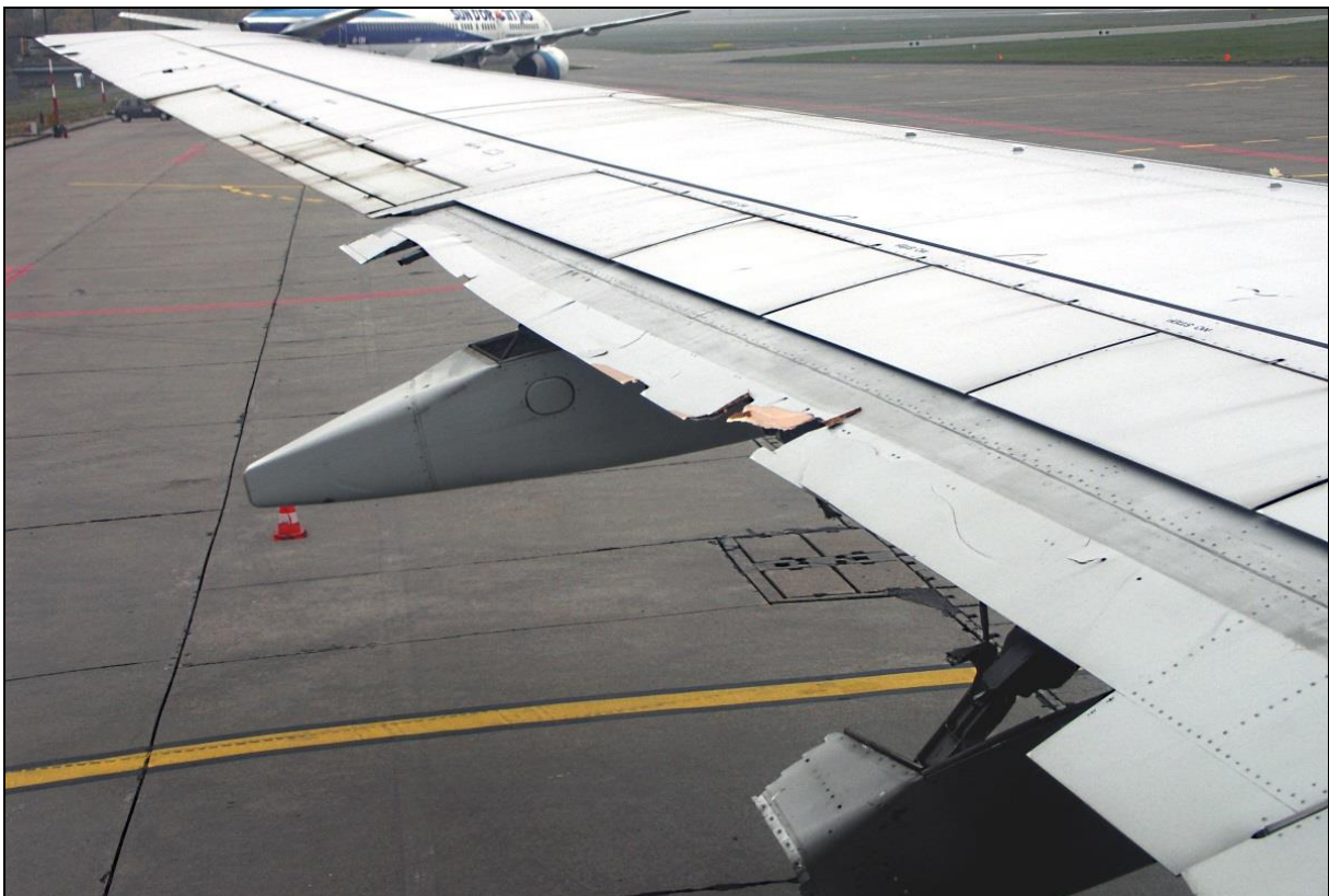
64 – Top view on the damaged left outboard flap. Visible part of the damaged track fairing
