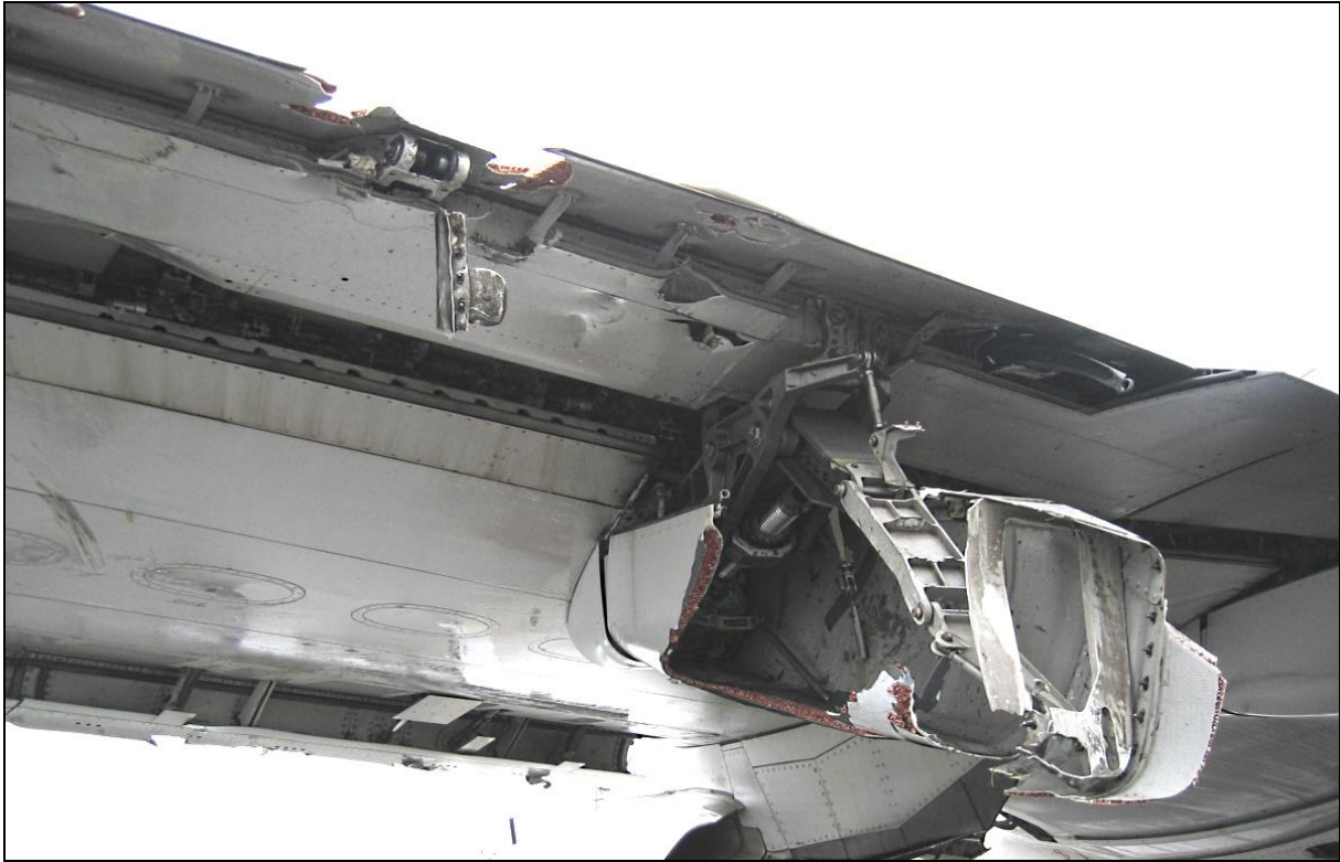
63 – Damage to the track fairing of the left outboard flap; visible damage to the flap [photo: airplane crew]
