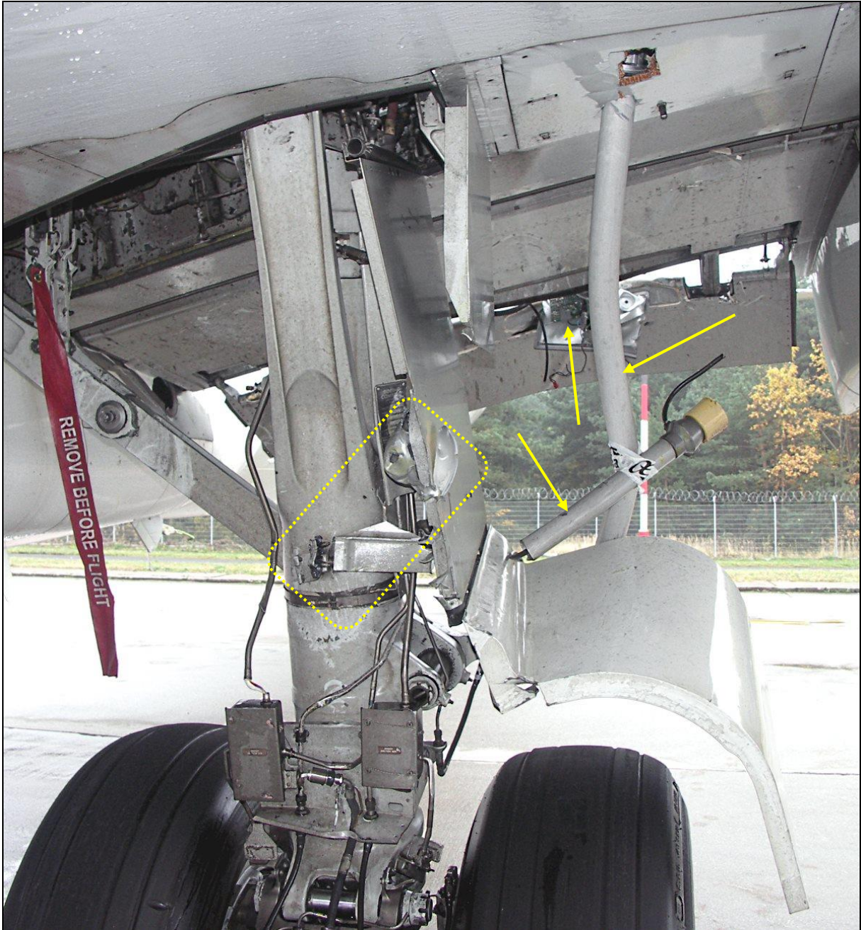
56 – Damage to the door of the left main landing gear and the bottom of the left inboard flap. Arrows show the lights pieces stuck in the airplane structure
