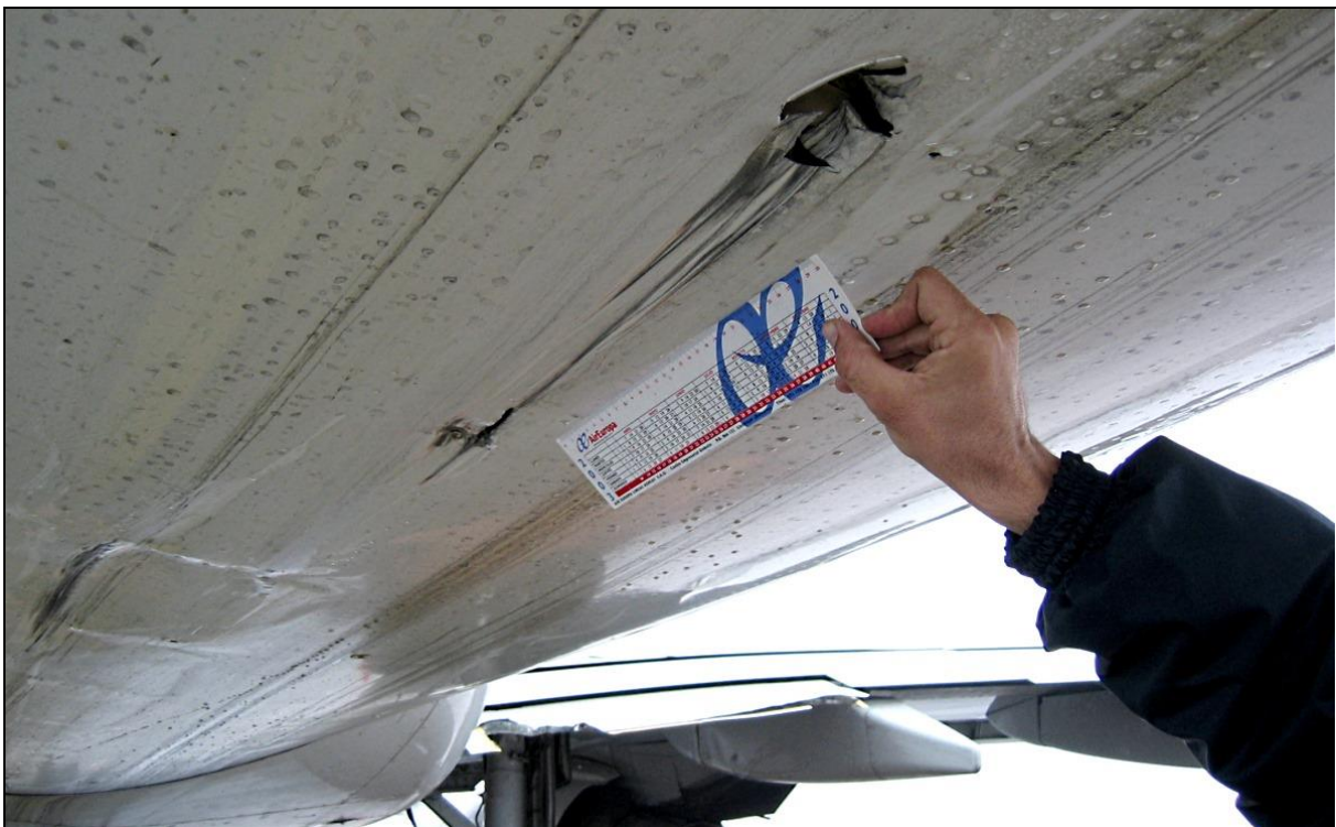
89 – Damage to the bottom part of the fuselage skin – close-up [photo: airplane crew]
