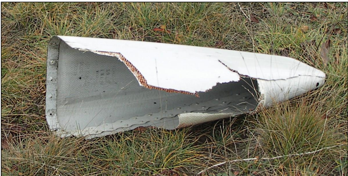
17 – Separated part of a flap track fairing from the left wing
