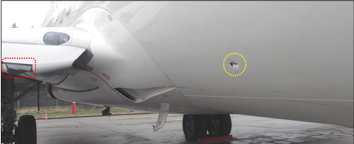
66 – Root area of the right wing – visible damage to the Krüger flap and fuselage puncture
