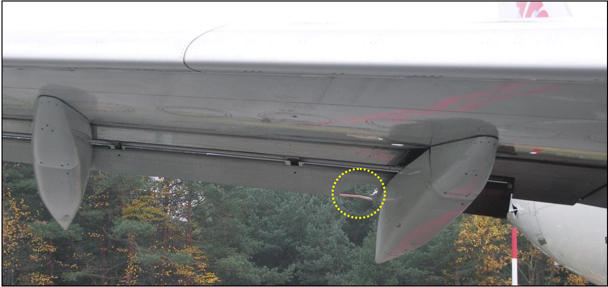
72 – Damage to the right outboard flap, bottom view
