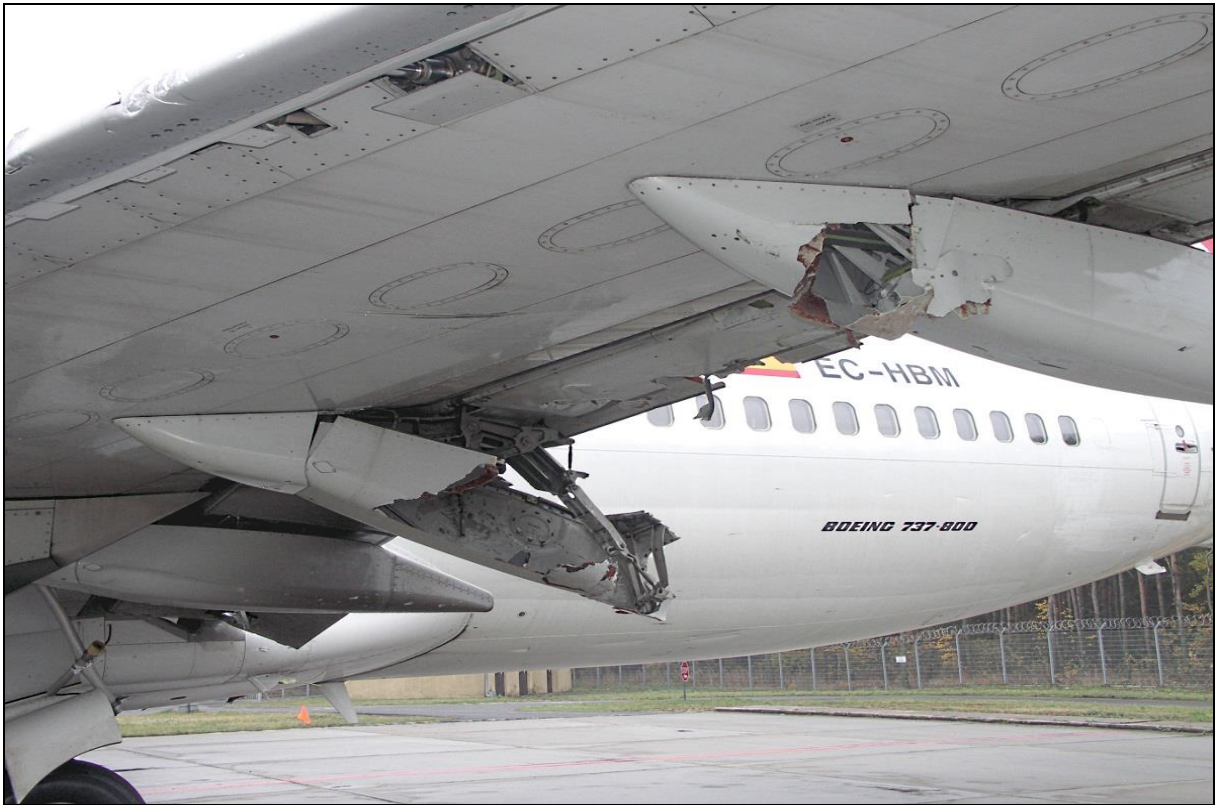
54 – Damage to the flap and flap track fairing of the left wing
