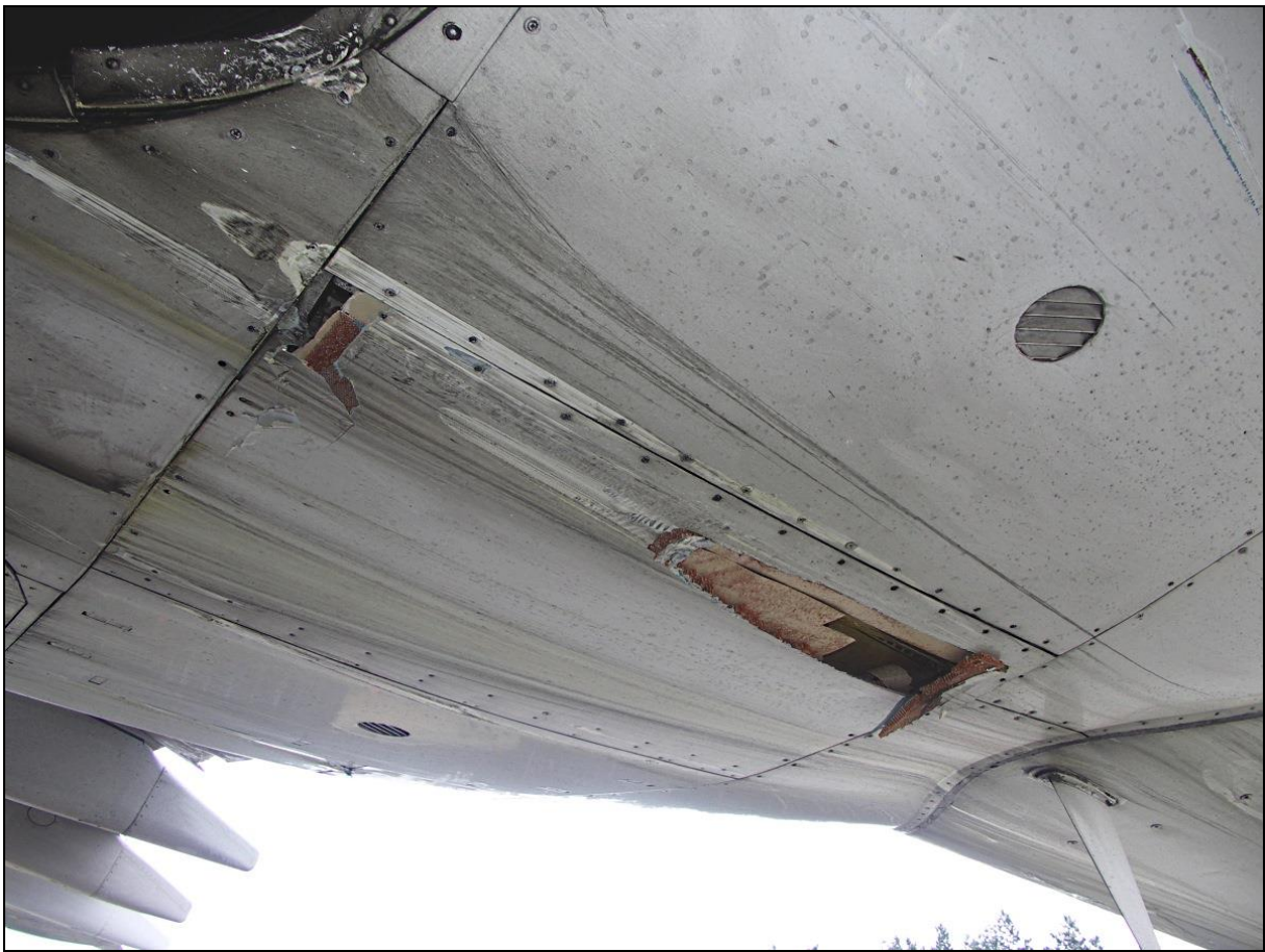
87 – Damage to the belly fairing – close-up
