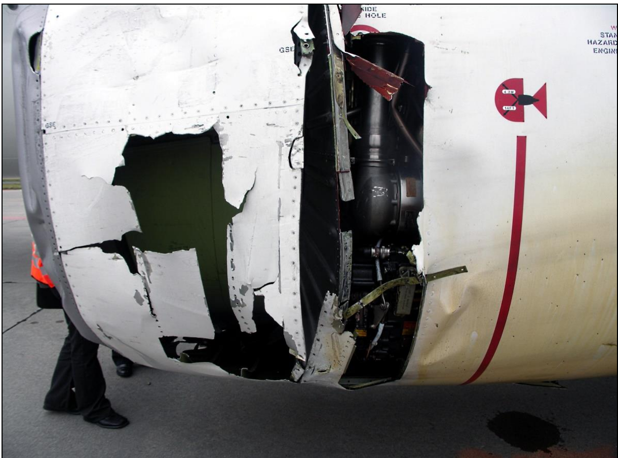
51 – Damage to the left side of the left engine nacelle
