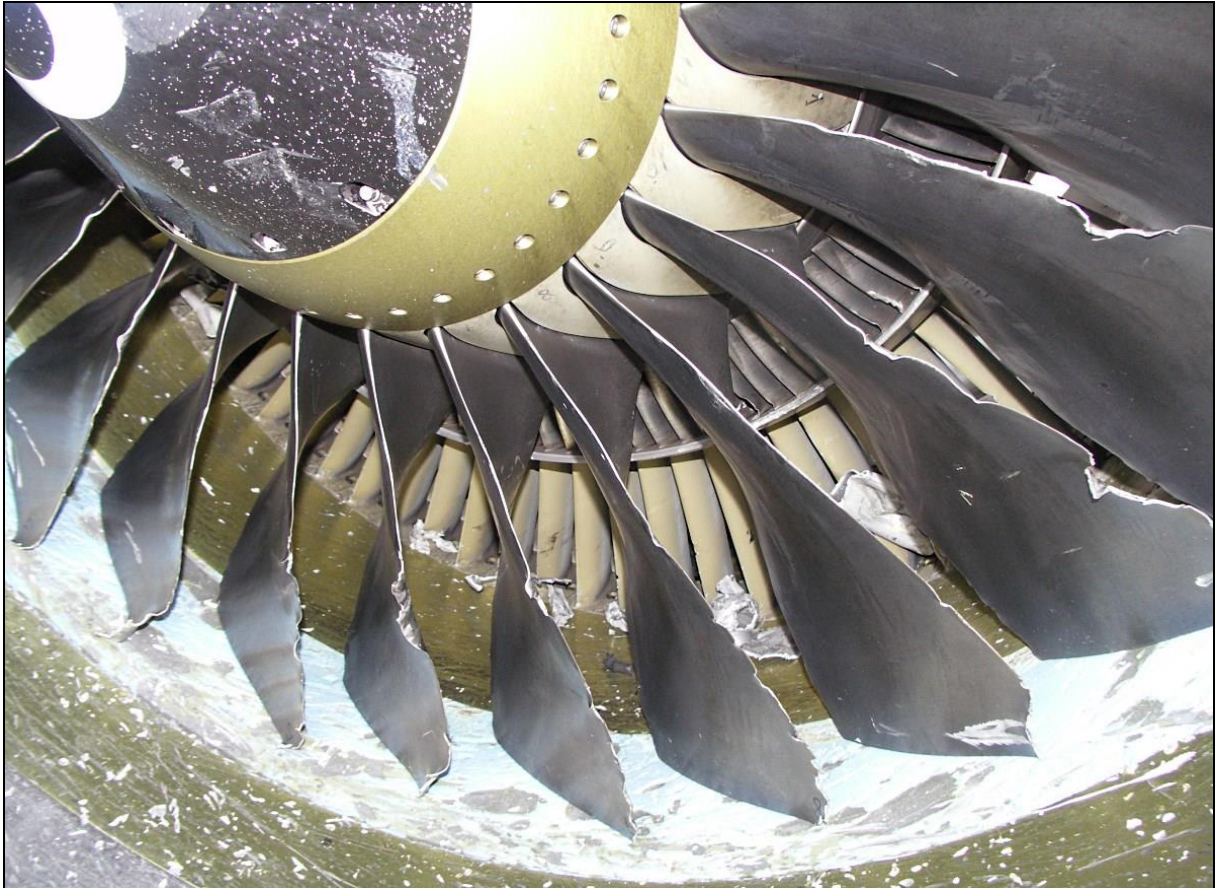
50 – Damage to the left engine fan – close-up
