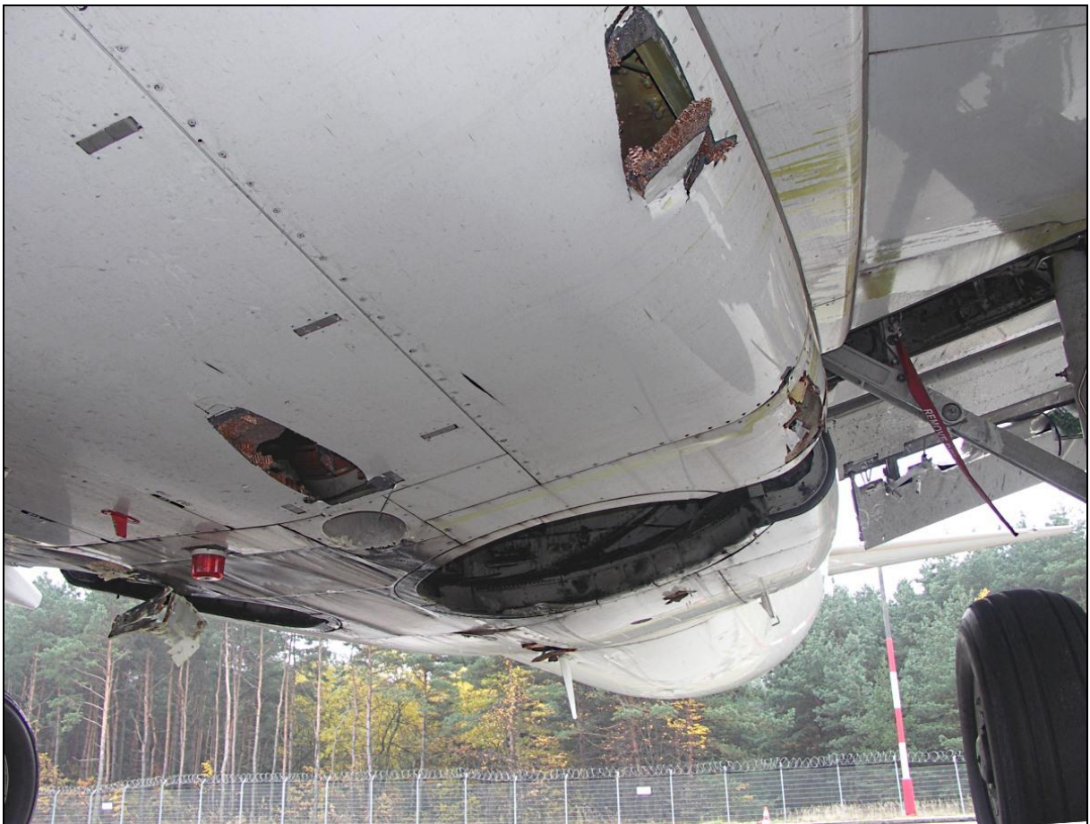
85 – Damage to the belly fairing – close-up [photo: airplane crew]
