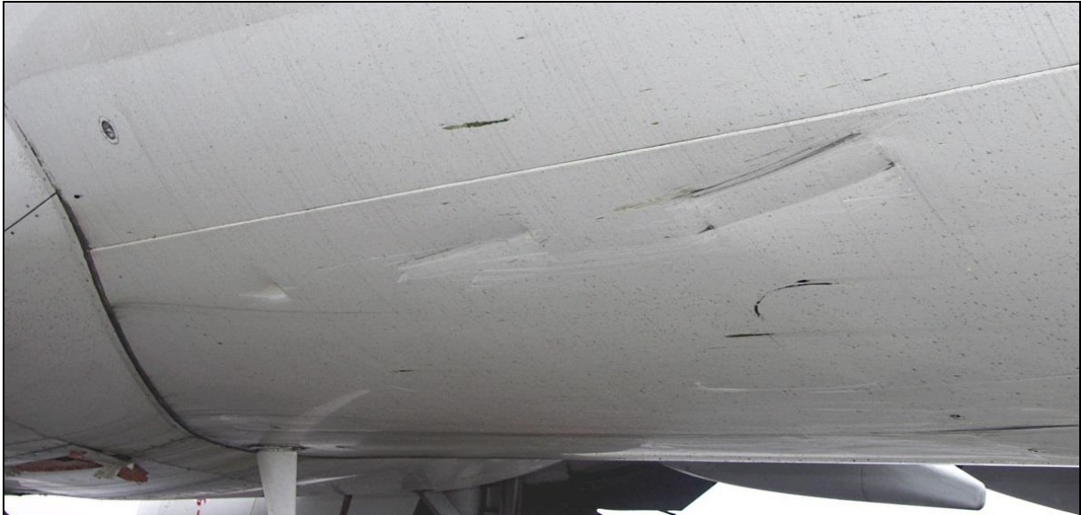
82 – Scratches and abrasions of the left rear part of the fuselage skin – close-up
