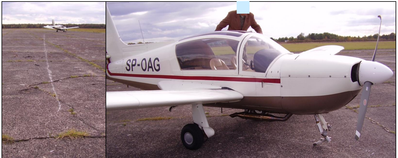
1, 2 – Landing track on a concrete and the airplane after coming to rest - attention is drawn to the lack of the nose landing gear wheel and damaged propeller. Photo T. Dunajski.
