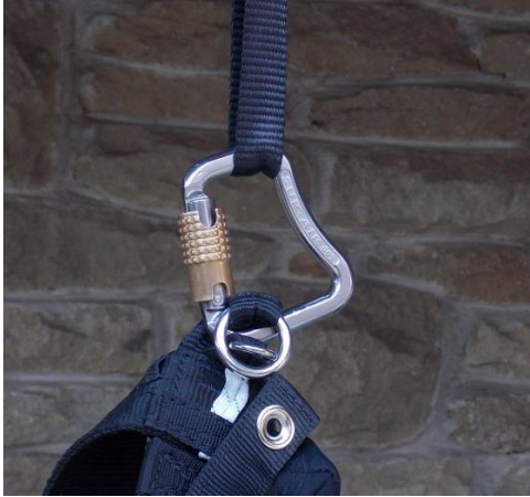
Photo 6. Different shape karabiner (SupAir - steel). The blocking of cut away process shows the same nature as in the case of SupAir aluminum karabiner - see photo 4.
