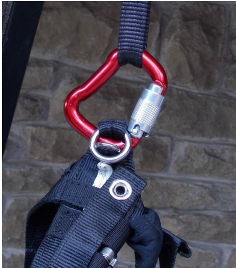
Photo 4. SupAir karabiner (aluminum) used in the accident flight. The blocking of cut away process was due to pressing on the small ring by the karabiner and blocking the movement of the bigger ring on the karabiner gate.
