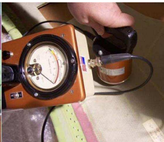
Figure 7 Moisture Meter used to determine location of moisture in Radome
