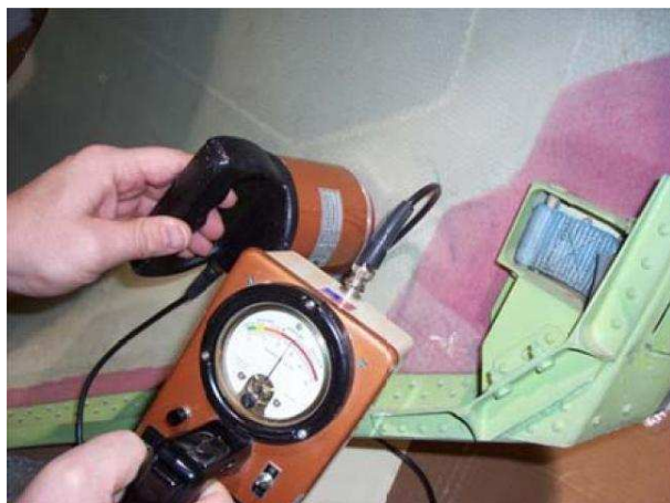
Figure 7 Moisture Meter used to determine location of moisture in Radome
