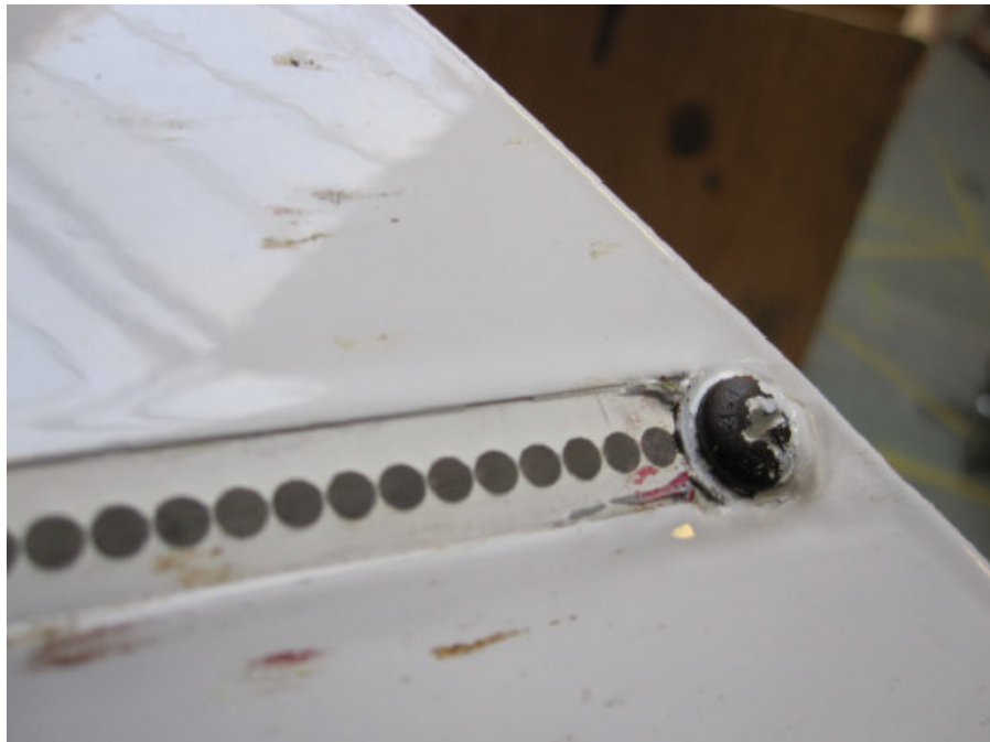
Deviating lightning diverter strip grounding/bonding Picture 10
