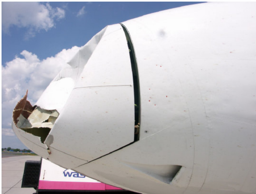
General view of the collapsed radome Picture 2
