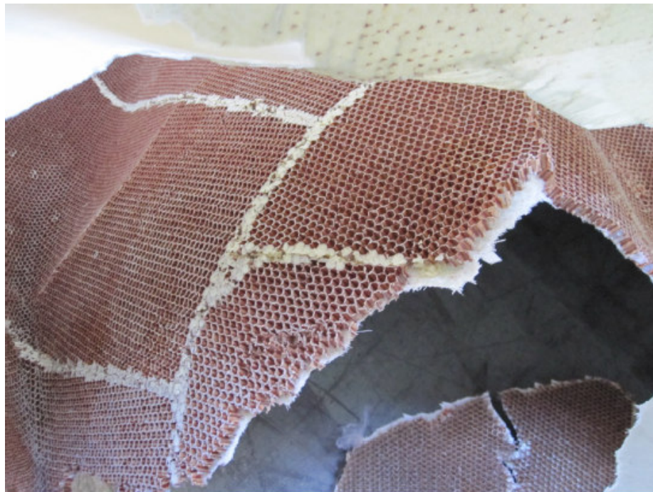
Details honeycomb core and inner skin plies Picture 6
