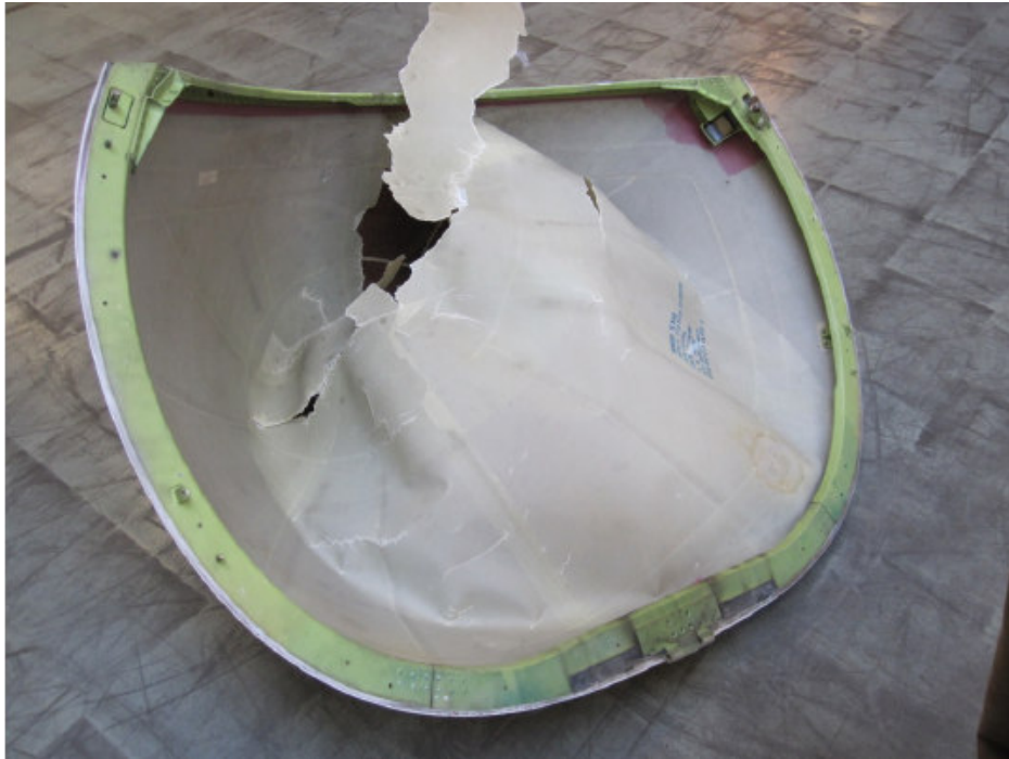
Delaminated inner plies Picture 8 (picture number according to the original)
