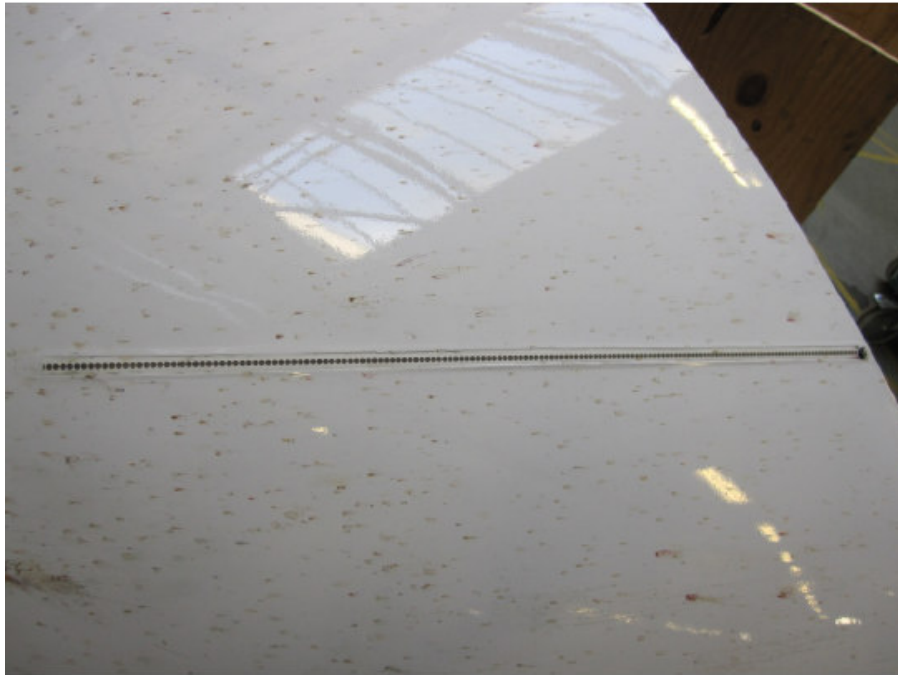
Deviating lightning diverter strip Picture 9
