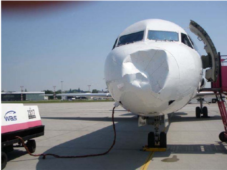
General view of the collapsed radome Picture 1
