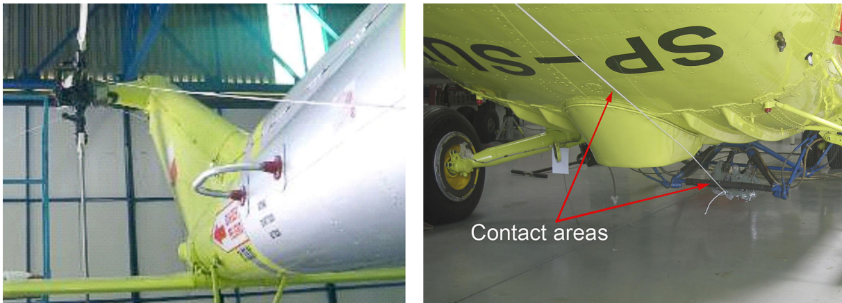
Figure 10. Photographs of the rope linking the load hook to the tail rotor on a helicopter of the same model as the accident helicopter
