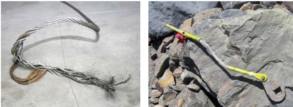
Figure 9. Photographs of the cable break. Top part at left and bottom at right
