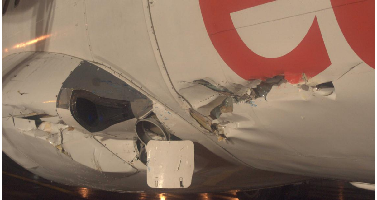
Photo 3. Damaged the landing gear gondola and the fuselage skin. (photo by LS Airport Service S.A.)
