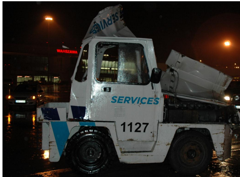
Photo 9. Damaged Mulag tractor with the side window opened. (photo by "Polish Airports" State Enterprise)
