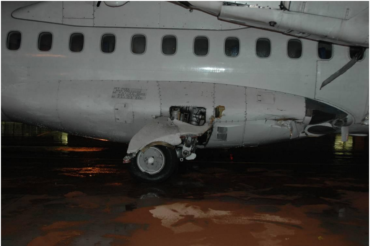
Photo 5. Damaged gondola of the right main landing gear (photo by “Polish Airports” State Enterprise)
