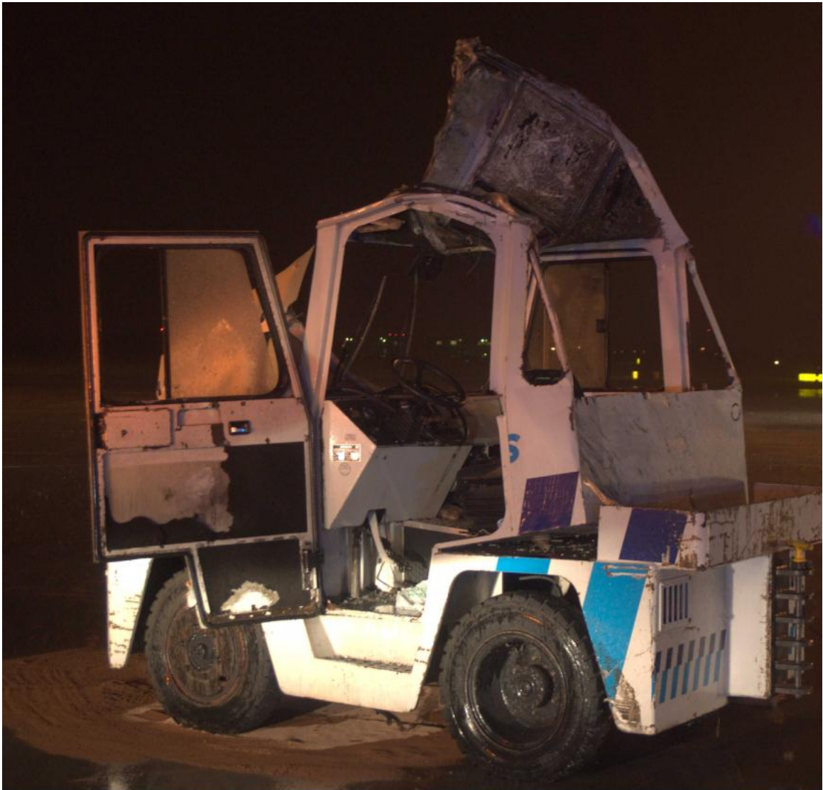
Photo 8. Rear cover damaged by the propeller (photo by LS Airport Service S.A.)
