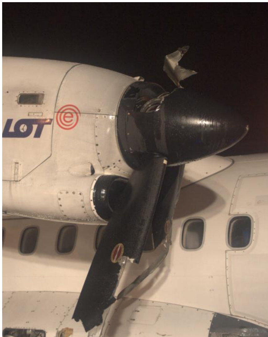
Photo 4. Damaged propeller. (photo by LS Airport Service S.A.)
