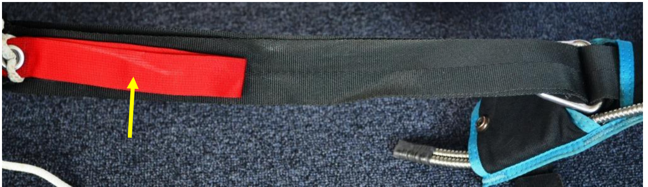
Photo 1. View of the back part of the right riser with a visible mark of melting on the back of the control handle. (Photo SCAA)
