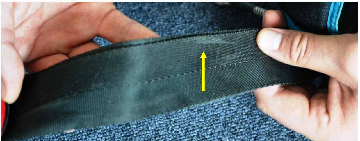
Photo 2. View of the back part of the left riser. Visible mark of melting. (Photo SCAA)
