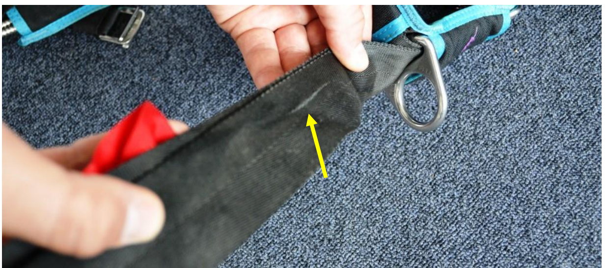
Photo 3. View of the front part of the left riser. Visible mark of melting. (Photo SCAA)
